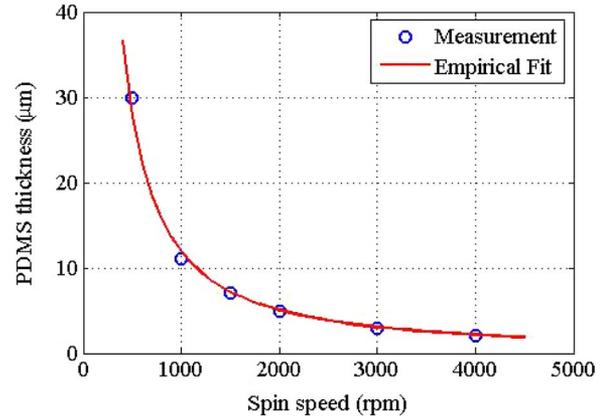
Fig. 5. PDMS thickness as a function of spin speed.
