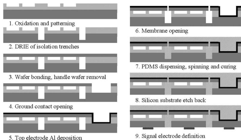
Fig. 6. Fabrication steps to incorporate CMUT elements onto a flexible silicon substrate.
