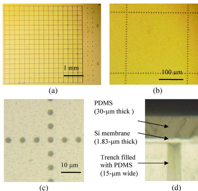
Fig. 7. Device photographs. (a) Front side view. (b) Magnified view of a single element. (c) Magnified view of through-wafer PDMS dispensing holes. (d) Cross-sectional view showing the trench, the membrane, and the PDMS coating and filling.
