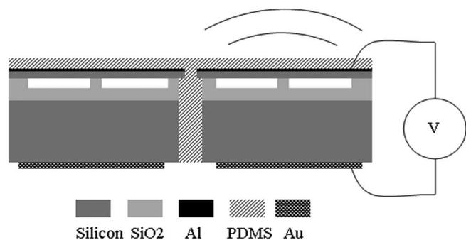
Fig. 2. Cross-sectional schematic of two flexible CMUT array elements. One of the elements is excited to transmit ultrasound waves into the surrounding medium.
