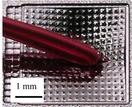
Fig. 9. Flexible 2-D CMUT array pushed by a wire on the back side.
