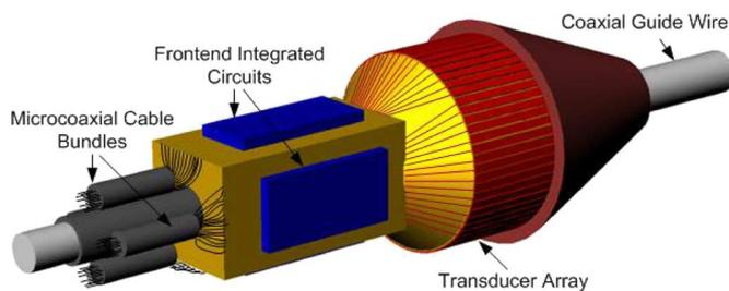
Fig. 1. Schematic of a catheter-based side-looking IVUS imaging probe (after [1]).
