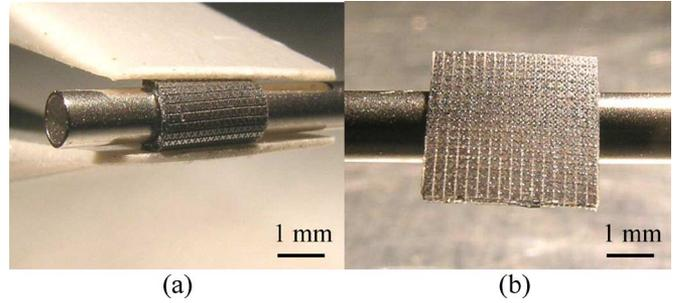
Fig. 4. Flexible silicon substrate realized by refilling through-wafer trenches with PDMS.
