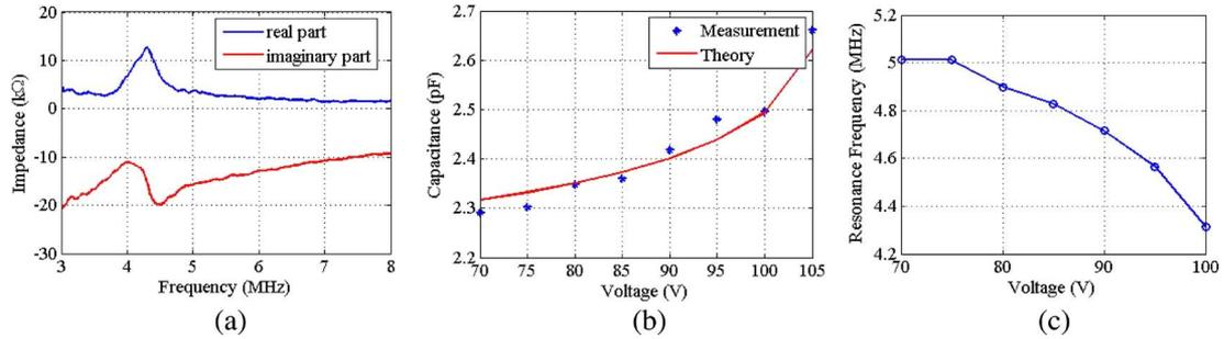
Fig. 8. Test results. (a) Electrical input impedance in air. (b) Device capacitance. (c) Resonant frequency.
