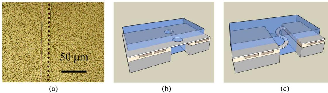
Fig. 10. (a) Photograph of cracks on the membrane. (b) Schematic of current dispensing hole design. (c) Schematic of proposed design to eliminate cracking.
