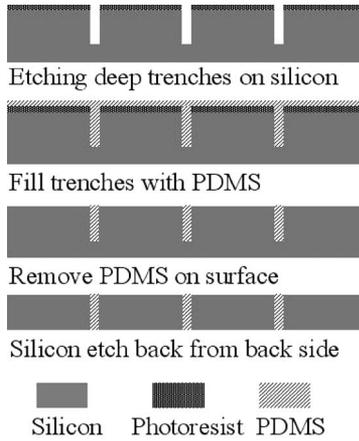
Fig. 3. Fabrication process to make a flexible silicon substrate by refilling through-wafer trenches with PDMS.
