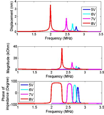
Figure 2. FEA result. Membrane displacement (top) and input impedance (bottom)
