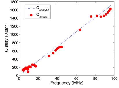
Figure 3.  $Q_{air}$  calculated from FEA and analytic method.
