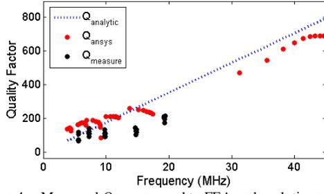
Figure 4. Measured  $Q_{air}$  compared to FEA and analytic method
