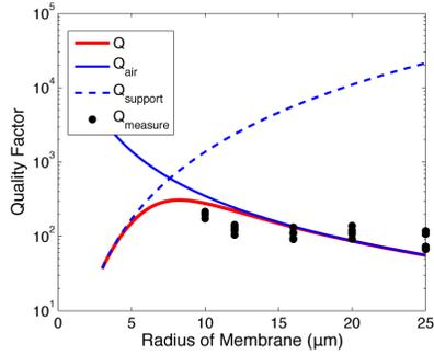
Figure 6. Estimated quality factor of silicon membrane of  $0.5 \mu\text{m}$  thickness and measured quality factor
