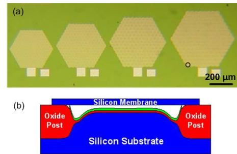
Figure 1. (a) Optical picture of CMUT. Circled area is single cell. (b) Schematic of cross section of single cell.
