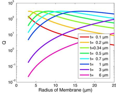
Figure 7. Estimated quality factor of silicon membranes with different thicknesses.
