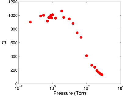
Figure 5. Measured quality factor in different pressure
