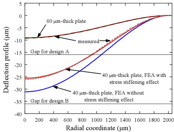
Fig. 2. Measured versus calculated plate deflection profiles for two designs A and B [7]. Design A has a deflection-to-thickness ratio of 65.2%, for B it is 15.2%.
