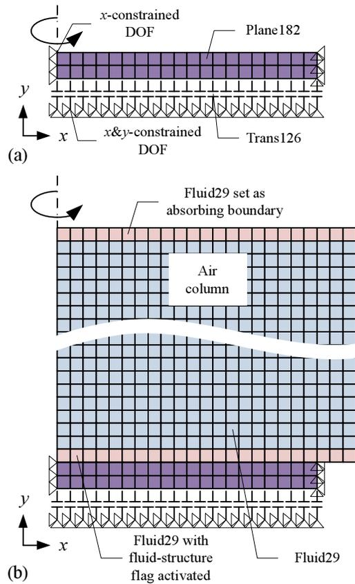
Fig. 1. Schematics of the two finite element models (FEMs) for the calculation of the static, modal, and harmonic response of circular CMUT plates, including stress stiffening effects.
