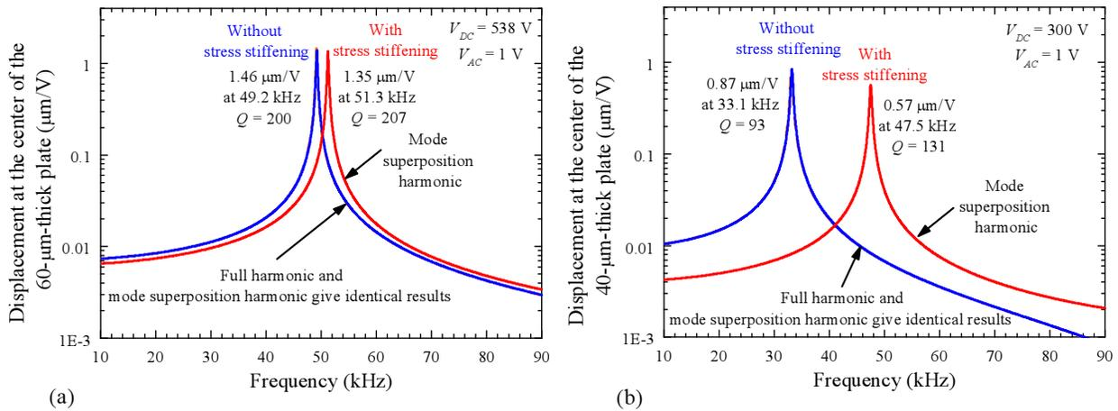
Fig. 5. Direct comparison for design B (left) and design A (right) of prestressed harmonic response analysis with linear static operation point calculation (blue) and prestressed mode superposition harmonic response analysis with nonlinear static operation point calculation (red).
