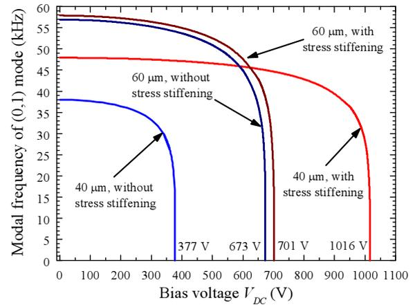
Fig. 4. Calculated modal frequency for mode (0,1) for design A and B as a function of the applied bias voltage  $V_{DC}$ .
