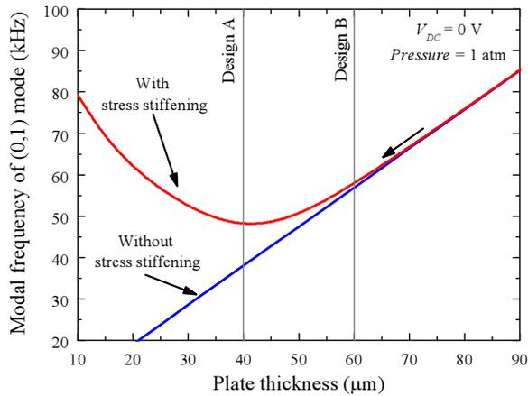
Fig. 3. Calculated modal frequency for mode (0,1) of a circular single crystal CMUT plate with a diameter of 4000  $\mu\text{m}$  as a function of its thickness.
