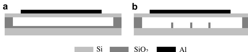
Fig. 1. Schematic cross-section of (a) conventional CMUT and (b) PostCMUT.
