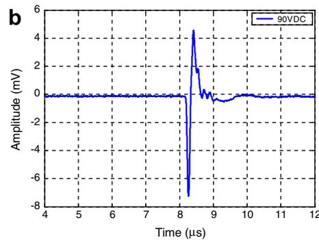
Fig. 9. Transmission pulses obtained by a hydrophone from a Conventional CMUT operating (a) before contact and (b) after contact. The input AC signal was a 5 V step function. Bias voltages are 40 V and 90 V for the measurements before contact and after contact, respectively.
