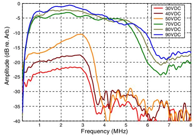
Fig. 10. Transmission spectrum (not corrected for medium attenuation or diffraction) of a Conventional CMUT at different bias voltages. The device operated in pre-contact region when the bias voltage is smaller than 50 V and in post-contact region when the bias voltage is larger than 70 V.
