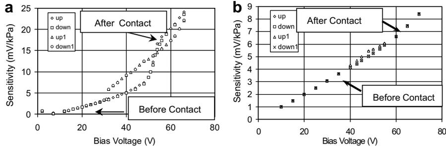
Fig. 5. Ultrasonic reception by CMUT as a function of bias voltage. Source: a PZT transducer with a constant output. (a) Conventional CMUT: hysteresis is evident after membrane-bottom electrode contact (collapsed region operation). (b) PostCMUT: good repeatability.
