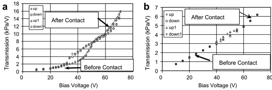
Fig. 6. Ultrasonic transmission by CMUT received by a broad band hydrophone as a function of bias voltage. (a) Conventional CMUT: hysteresis is evident after membrane-bottom electrode contact (collapsed region operation). (b) PostCMUT: good repeatability.
