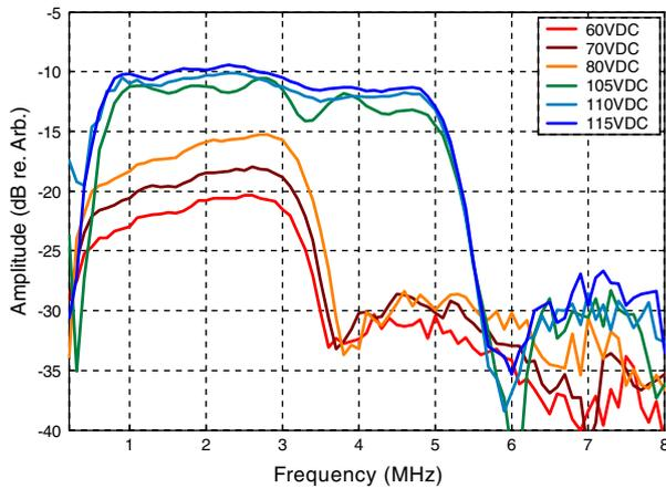
Fig. 8. Transmission spectrum (not corrected for medium attenuation or diffraction) of a PostCMUT at different bias voltages. The device operated in pre-contact region when the bias voltage is smaller than 80 V and in post-contact region when the bias voltage is larger than 105 V.
