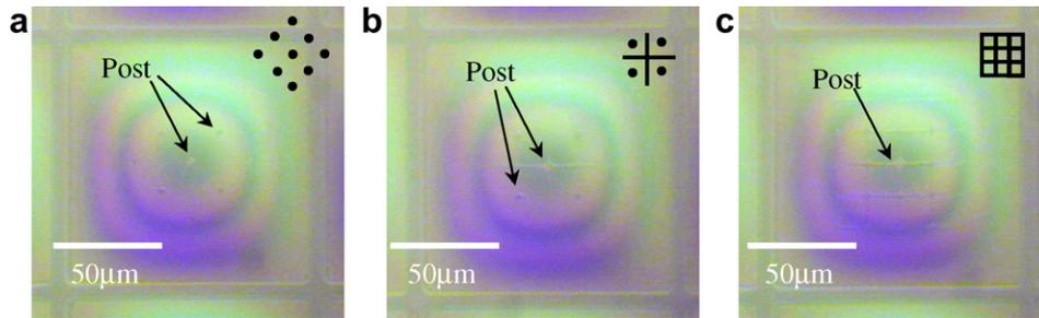
Fig. 3. Photographs of fabricated devices with different post patterns showed in the top right corners: (a) 9-point pattern (b) cross pattern and (c) net pattern.
