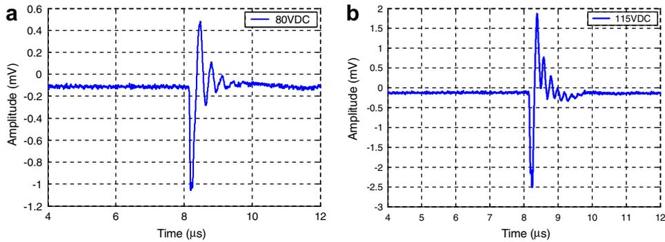
Fig. 7. Transmission pulses obtained by a hydrophone from a PostCMUT operating (a) before contact and (b) after contact. The input AC signal was a 5 V step function. Bias voltages are 80 V and 115 V for the measurements before contact and after contact, respectively.
