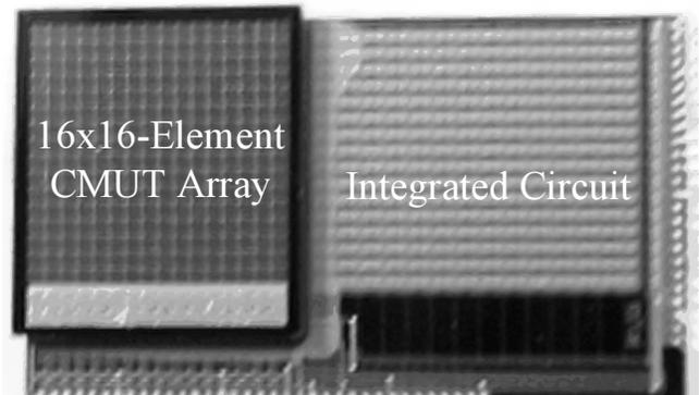
Fig. 4. A photo of a CMUT array flip-chip bonded to the integrated circuit.
