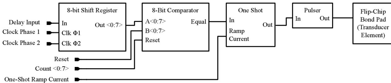
Fig. 2. Transmit circuitry is provided to each of the 224 transmitting elements. Prior to transmit, a delay value is loaded into the 8-bit shift register. The pulser is triggered when the stored value is equal to a global counter. A one-shot determines the width of the pulse.
