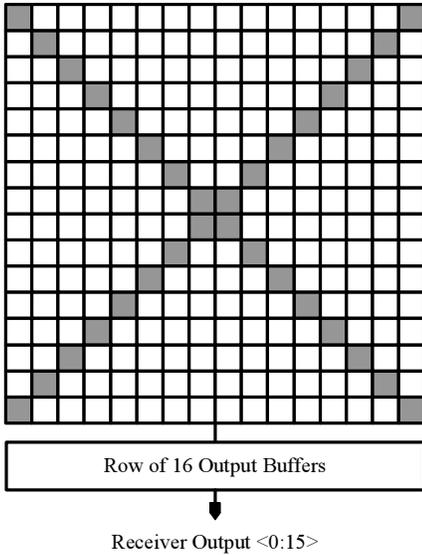
Fig. 1. The IC uses the 32 elements along the array diagonals to receive. A preamplifier is provided to each of the receiving elements. The remaining elements are used to transmit. The transmit circuitry includes shift registers that store delay information so that all of the transmitting elements can be used in parallel to transmit focused ultrasound.
