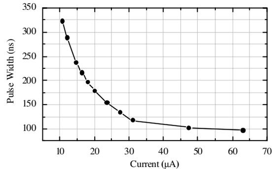
Fig. 6. A control-current for the one-shot is used to adjust the pulse width.
