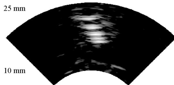
Fig. 7. A two-dimensional image of a nylon-wire phantom was acquired. The image is shown with 25-dB dynamic range.
