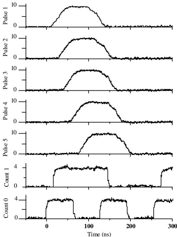
Fig. 5. The output of 5 pulser along with two bits of the global Gray code counter are shown. In this case, the pulser's shift registers are loaded with values such that the pulser's fire in succession as the Gray code counter is incremented. Each transition of Count 0 corresponds to 4 increments of the total Gray code counter value.
