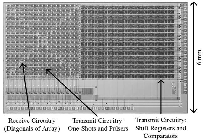
Fig. 3. A photo of the fabricated integrated circuit.
