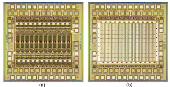
**Figure 2.** (a) Photograph of the custom-designed front-end electronics, (b) Photograph of a CMUT ML array flip-chip bonded to the front-end electronics.
