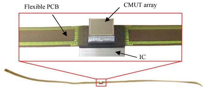
**Figure 6.** A photograph of the front-end IC and the CMUT ML array flip-chip bonded to two sides of the flexible PCB for final catheter assembly.
