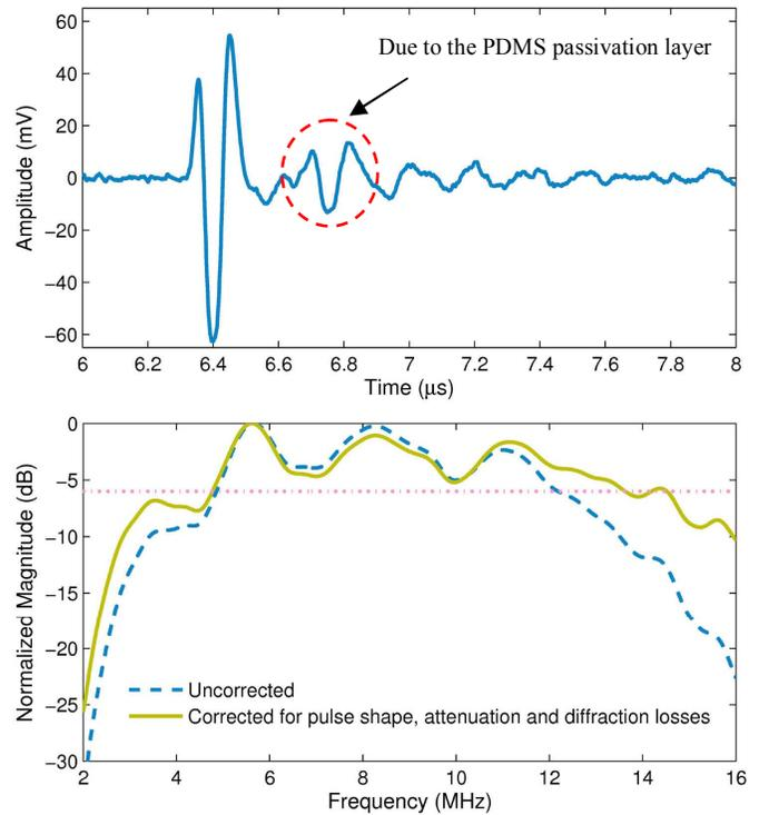
**Figure 4.** The pulse echo and its frequency spectrum from an element of the CMUT ML array immersed in water at a 4.7 mm depth. The device was biased at negative 30 V. The second echo in the top figure is because of the rather large impedance mismatch between the PDMS layer and water.
