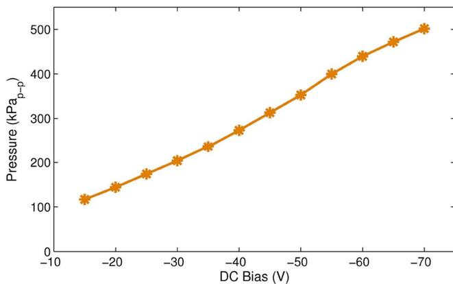
**Figure 3.** Acoustic peak-to-peak pressure at the face of the ML array as a function of DC bias. The AC pulse amplitude was 24 V.
