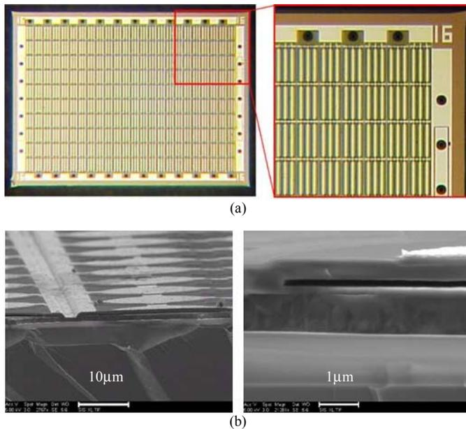
**Figure 1.** (a) Optical picture of a CMUT ML array composed of rectangular membranes, (b) SEM pictures of a CMUT ML array with circular membranes.
