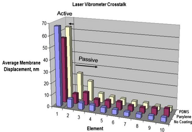
**Figure 6.** Crosstalk measurement results using a Polytec laser vibrometer.
