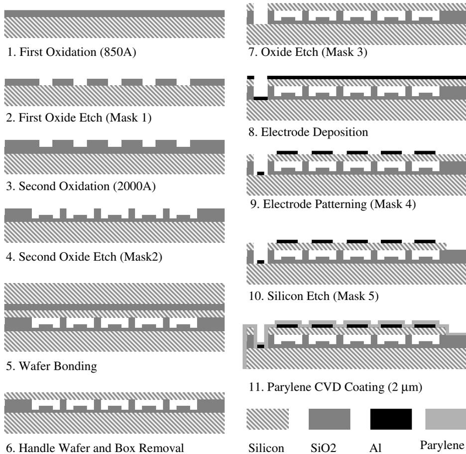
**Figure 3.** CMUT device fabrication diagram using a SOI wafer bonding process.
