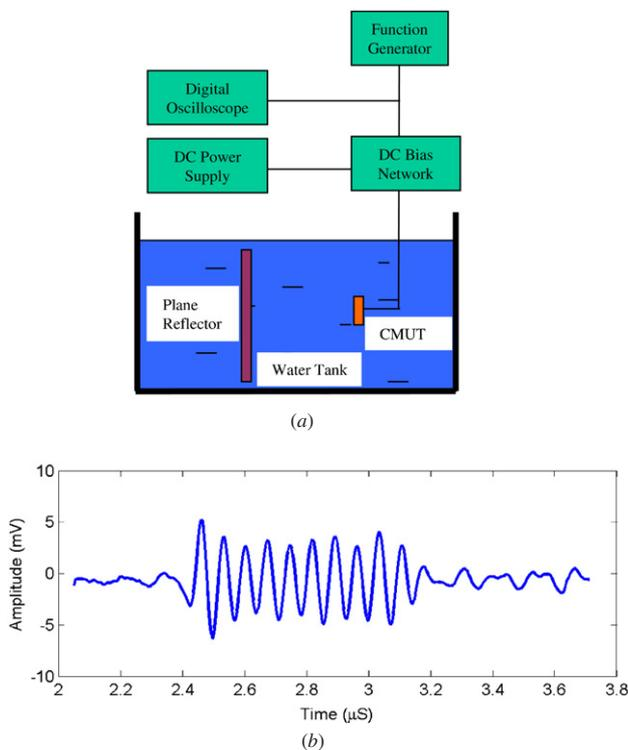
**Figure 7.** (a) Schematic of experimental setup for pulse-echo measurement. (b) Received echo signal in water.
