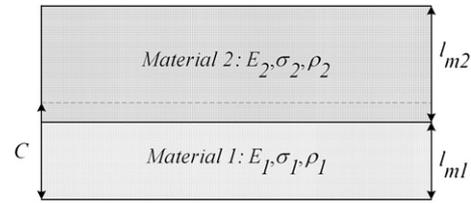
**Figure 2.** A schematic of a compound plate composed of two different materials.
