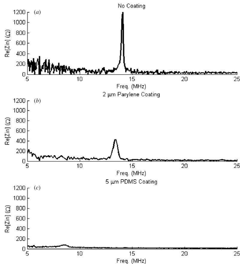
**Figure 5.** Effects of parylene and PDMS coatings on the real part of the input impedance of a device with 48  $\mu\text{m}$  diameter circular membranes. (a) The peak amplitude is  $\sim 1200\ \Omega$  (b) the peak amplitude decreases to  $\sim 480\ \Omega$  and (c) the peak amplitude decreases to  $\sim 100\ \Omega$ .
