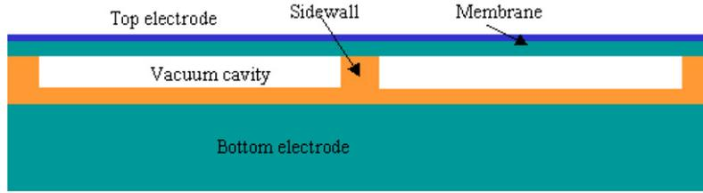
**Figure 1.** Cross section of two CMUT cells connected in parallel.
