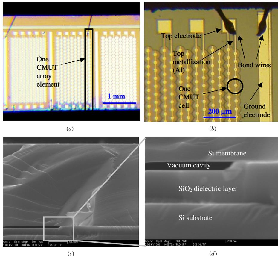
**Figure 4.** Device pictures of (a) three different CMUT arrays, (b) a close-up of one array showing bond wires to both the top and bottom electrodes, (c) SEM cross-sectional view of a CMUT cell without coatings and (d) zoom in of (c) showing the membrane, cavity and dielectric layers.
