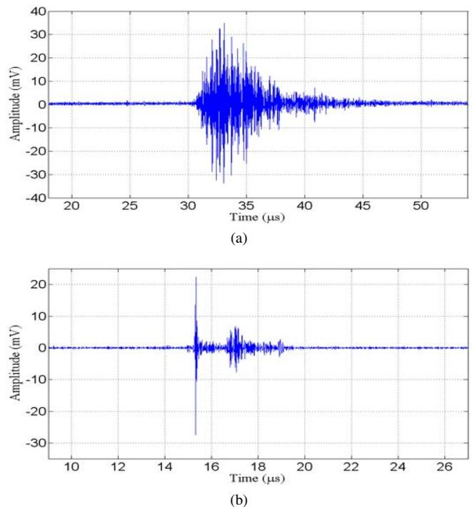
Fig. 6. Sample A-scans from the pig kidney, taken from the same spot: (a) Pulse-echo a-scan (b) Photoacoustic a-scan
