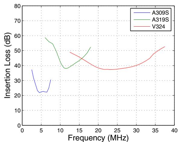
Fig. 2. 2-way insertion loss measurement of Panametrics transducers.
