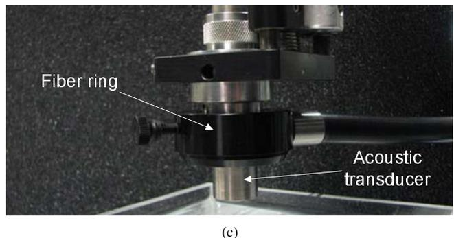
Fig. 1. Experimental setup: (a) Labeled schematic of setup (b) Photograph of setup (c) Transducer holder and fiber ring close up
