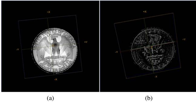
Fig. 3. Pulse-echo images of a United States quarter dollar coin: (a) Top surface of coin, 25dB (b) Bottom surface of coin with focus of transducer still on top surface of coin, 25dB
