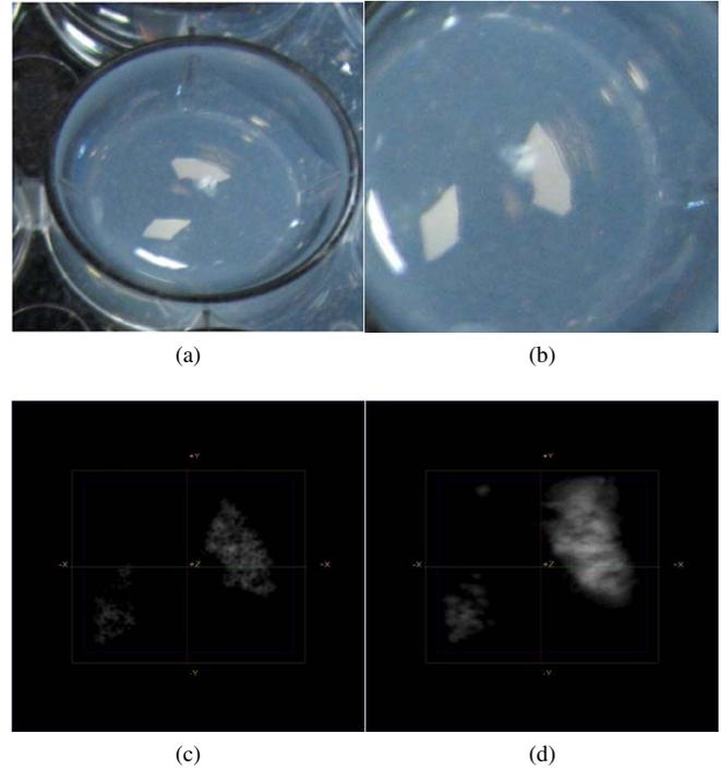
Fig. 5. Images of eggshell fragments in agar gel: (a) Photograph of eggshell fragments in agar gel (b) Zoomed in photo of eggshell fragments (c) Pulse-echo image, 30 dB (d) Photoacoustic image, 30 dB
