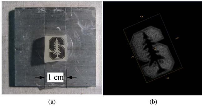
Fig. 4. Printed Stanford logo phantom: (a) Photograph of Stanford logo phantom (b) Photoacoustic image of Stanford logo phantom, 25 dB
