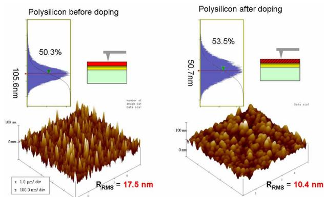
Fig. 6: Doping reduces surface roughness of polysilicon
