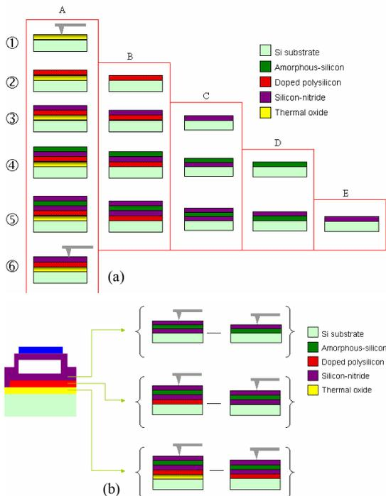
Fig. 2: The methodology to quantify the roughness of each layer
