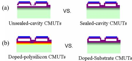
Fig. 1: The comparison of the surface roughness from the bottom side of the gap between (a) The CMUTs with and without sealing, and (b) The CMUT with doped polysilicon and thermal oxide and the one with doped substrate
