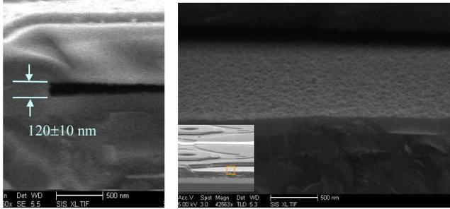
Fig. 4: (a) SEM photograph (cross-section) of one CMUT cell showing the gap-height, and (b) SEM photograph of surface roughness from the bottom side of the gap
