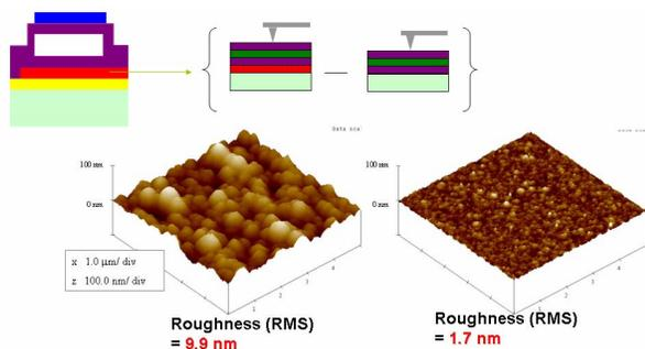
Fig. 7: Roughness contributed from doped polysilicon
