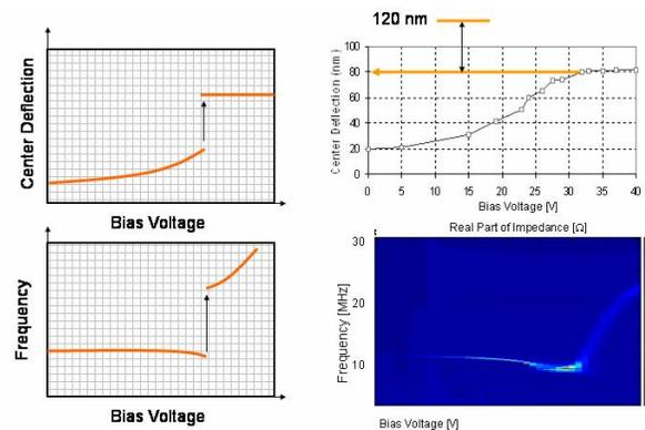
Fig. 3: Behavior of center deflection versus DC bias and real part of input impedance versus DC bias: (a) Theoretical part, and (b). Measurements part.
