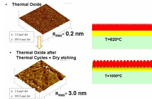
Fig. 5: Thermal Oxide is roughened due to imprinting by overlying polysilicon layer
