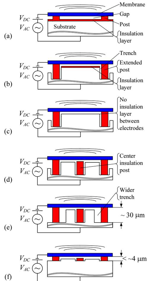
Fig. 1. Schematic of a traditional capacitive ultrasonic transducer cell (a) in direct comparison to various improved cell configurations (b)-(f). Red is an insulating material, such as silicon dioxide, blue is preferentially conductive, such as doped silicon or silicon carbide (for CMUT, top electrode is then optional) or a metal foil (for CUT). If the membrane (blue) is non-conductive (e.g. silicon nitride, nanocrystalline diamond film) then a top electrode is required (not shown).
