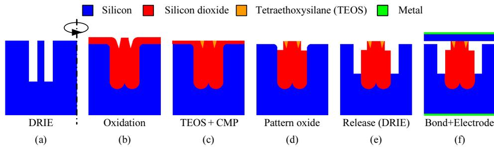
Fig. 2. Key steps of the fabrication process to realize a released  $\sim 4 \dots 30 \mu\text{m}$ -deep thermally-grown  $\text{Si}_2\text{O}_2$  insulation structure. Each figure (a-f) shows the cross section of a circular shaped structure.
