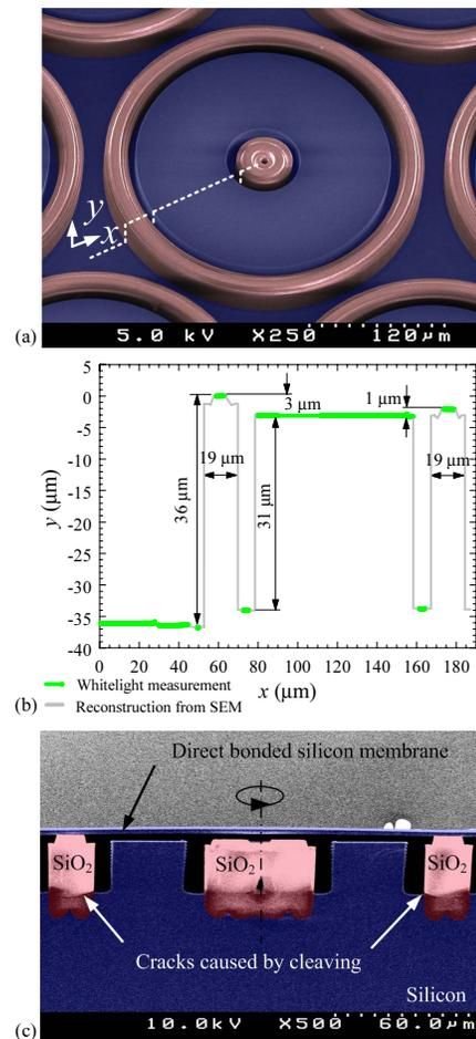
Fig. 3. Fabrication results: (a) Colorized SEM photograph (red...solid silicon dioxide, blue...heavily doped silicon) after the release step of one exemplary configuration fabricated. The dashed line outlines the location of the white light profiler measurement, shown in (b). (c) Colorized SEM photograph of an exemplary cross-section (cleaved sample) after direct wafer bonding to an SOI wafer. The handle wafer and box-layer have been removed.
