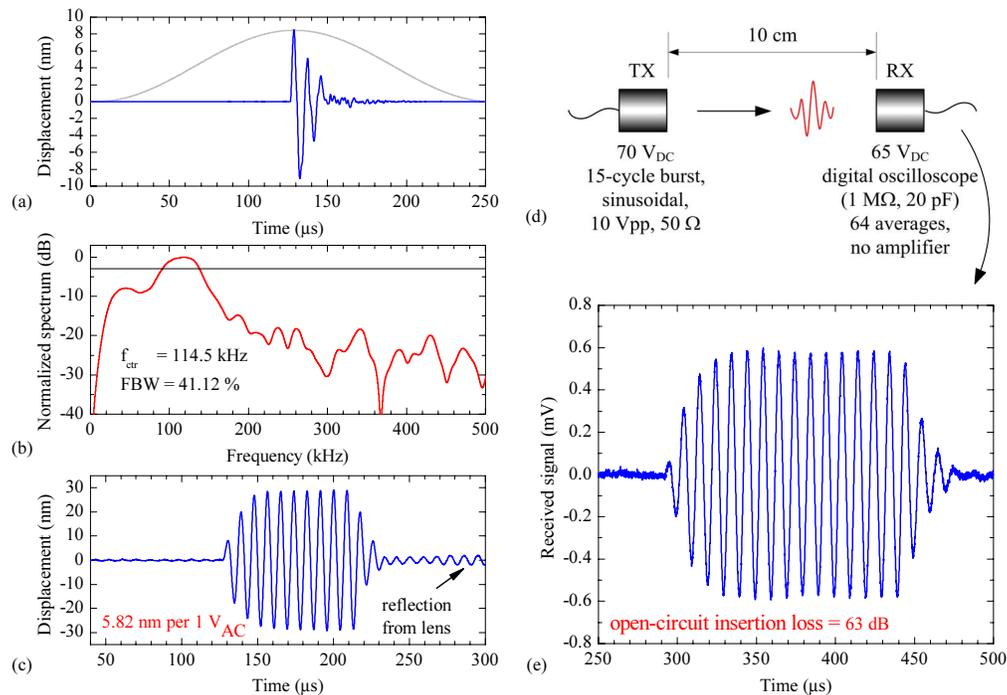
Fig. 4. Preliminary characterization results from a capacitive ultrasonic transducer featuring the back plate shown in Fig. 3(a). Impulse response (displacement) in time (a) and frequency domain (b) of a single cell. Response of a single cell to a 10-cycle sinusoidal burst signal at a center frequency of 114.5 kHz (c). Pitch-catch configuration (d) and measured received signal (e).
