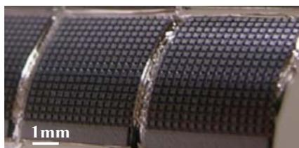
Figure 8: Trench-isolated 2D CMUT arrays with a curvature.
