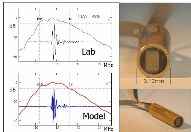
**Figure 3.** The measured and KLM model performance of the 2<sup>nd</sup> generation forward-looking PZT array, mounted on the inside of the flex circuit bend.
