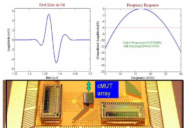
**Figure 4.** The pulse echo and spectral response from the 24 element cMUT array emerged in oil at a 1mm depth. A 60VDC bias and 24V pulses were used with a transimpedance amplifier configuration.
