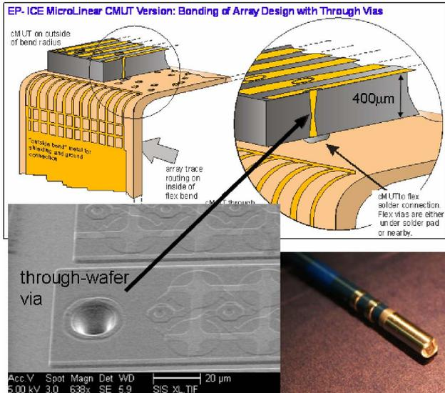
**Figure 2.** The position of the cMUT array mounted on the folded flex circuit is shown at the top with the unique through-wafer via to allow top trace communication with the flex pads. The lower right is a mock-up of the final assembly with metal tip enclosure.
