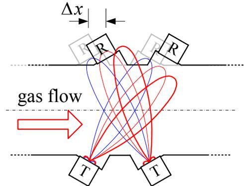
Fig. 1. A double-path UFM extended in its rangeability by shifting both receiving transducers (R) by the same shift distance ( $\Delta x$ ) in flow direction to compensate for the carry-along effect (sound drift).
