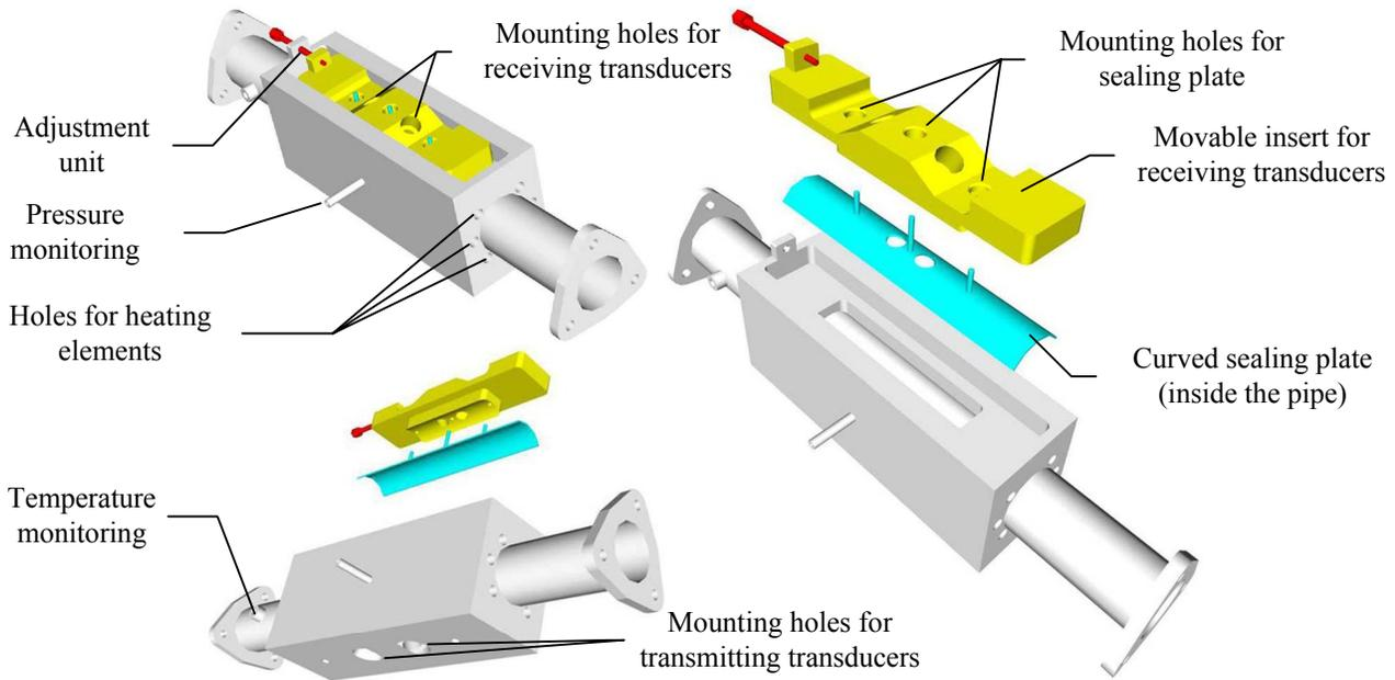
Fig. 2. Design drawings (different views) to illustrate the realization of an adaptive asymmetric UFM. The movable insert enables shifting both receiving transducers with and against the flow direction during UFM operation. The curved sealing plate is mounted inside the pipe. (Drawing by courtesy of AVL List GmbH, Graz, Austria.)
