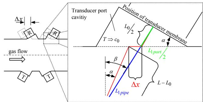
Fig. 3. Schematic of how the shift distance ( $\Delta x$ ) and transducer port cavities are considered for the derivation of the UFM equations ( $v$ ,  $c$ ) for the asymmetric configuration.
