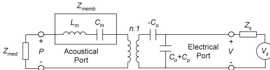
Figure 3: CMUT equivalent circuit in transmit.
