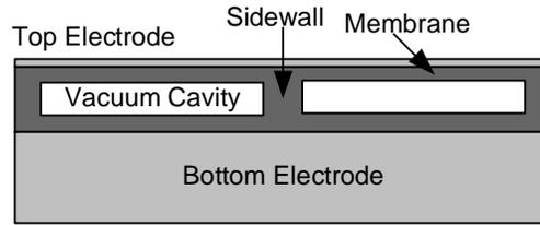
Figure 1: A simplified schematic of a CMUT.
