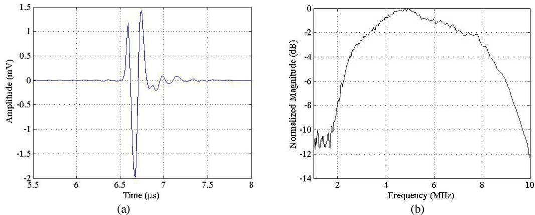
Figure 8: (a) Response of the CMUT to a pulse excitation in vegetable oil, (b) Fourier transform of the response, corrected for medium attenuation, diffraction, and hydrophone response.
