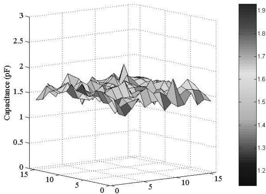
Figure 7: Total capacitance distribution across a 2D CMUT array.
