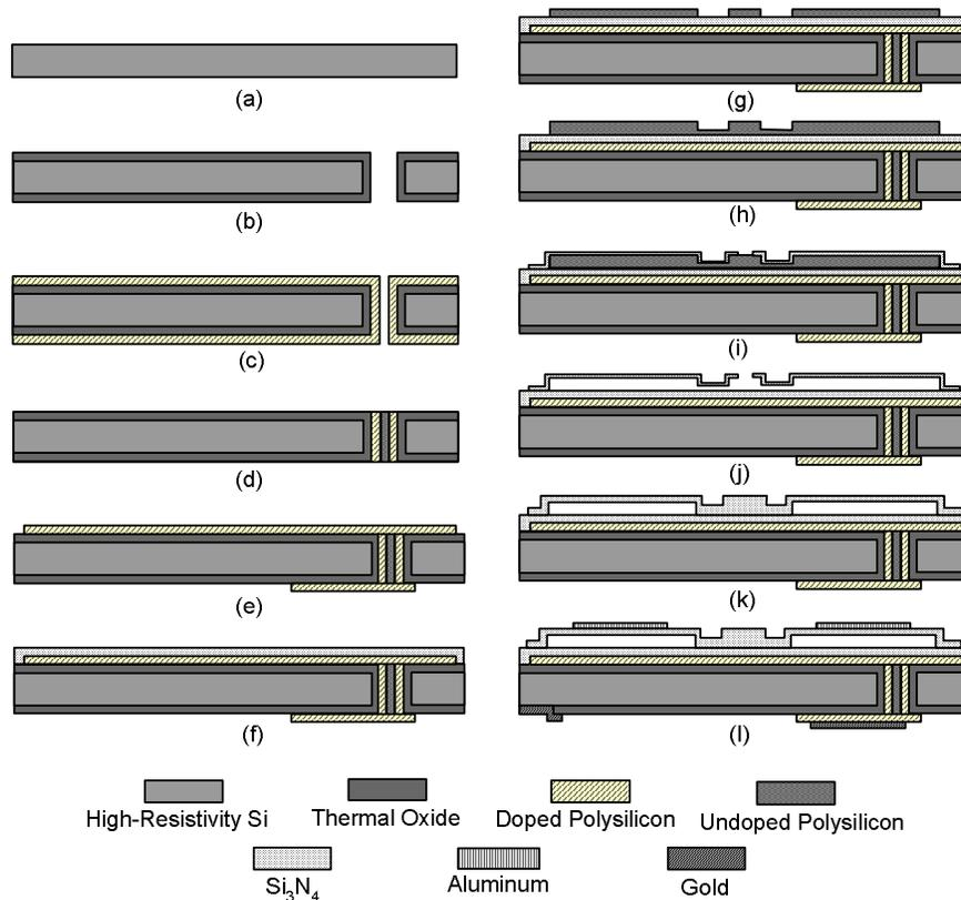
Figure 4: Process flow of CMUT fabrication.
