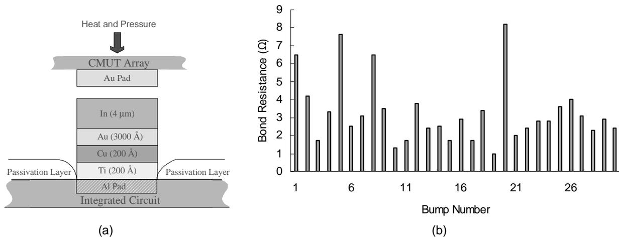
Figure 13: (a) Metal stack used for flip-chip bonding, (b) bond resistance.
