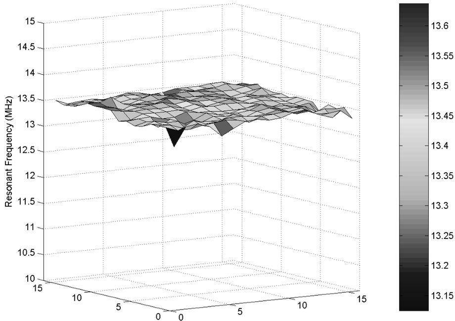
Figure 6: Resonant frequency distribution across a 2D CMUT array.
