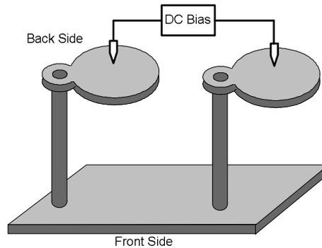
Figure 12: Schematic of series resistance measurement setup.
