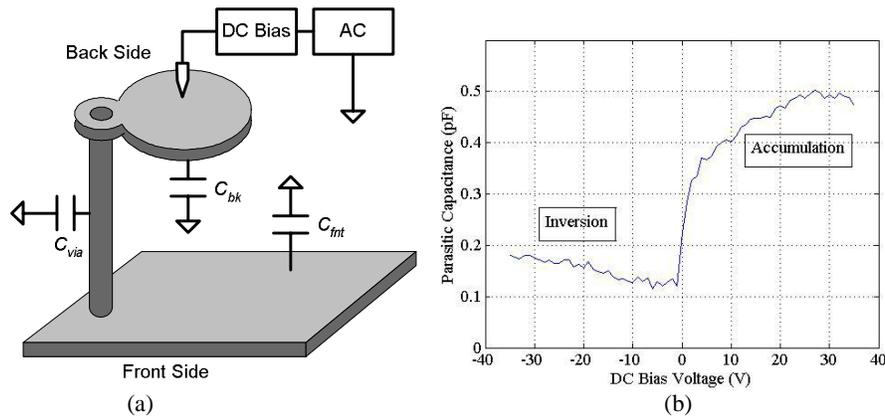
Figure 11: (a) Schematic of the parasitic capacitance measurement setup, (b) parasitic capacitance as a function of DC voltage.
