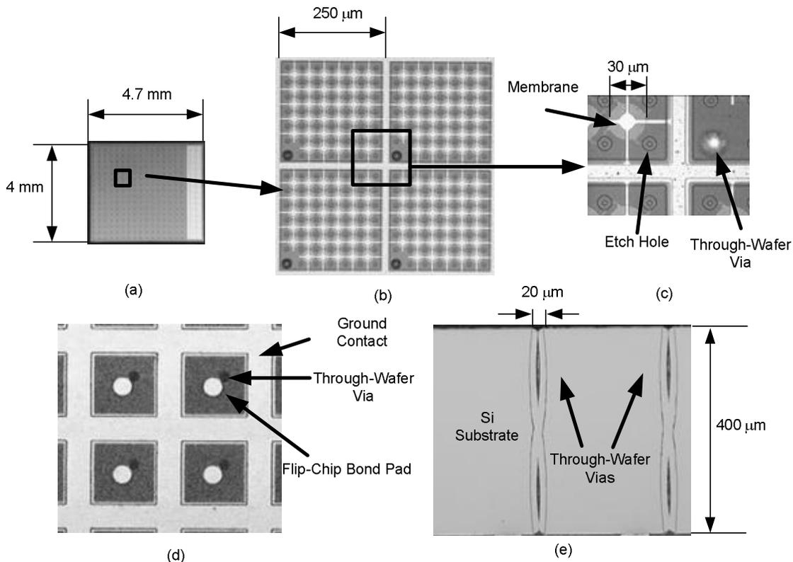
Figure 5: Pictures of a 2D array, array elements and through-wafer vias.
