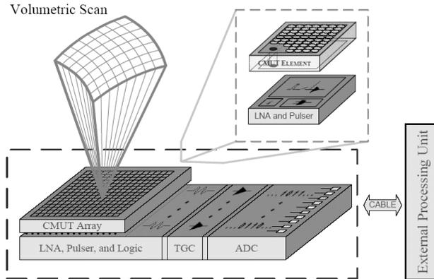
Figure 2: Miniature real-time volumetric imaging system based on 2D CMUT array.
