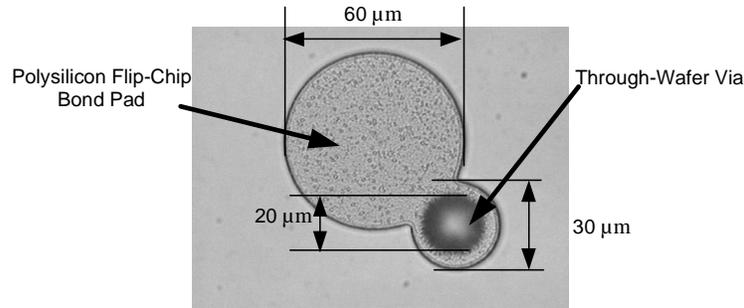
Figure 10: Picture of a polysilicon pad with minimal area.
