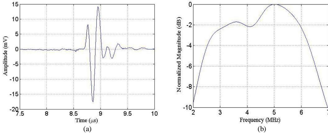
Figure 9: (a) Pulse-echo measurement of the CMUT with custom IC, (b) uncorrected Fourier transform.
