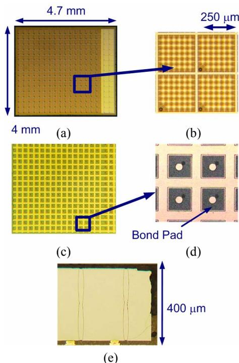
Figure 3. Photographs of the fabricated arrays. (a) Top side. (b) Close-up of 4 elements. (c) Back side. (d) Back side of 4 elements showing the through-wafer vias. (e) Cross section showing the through-wafer vias.
