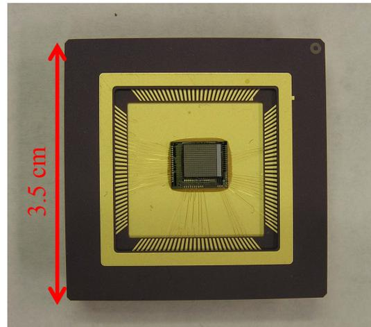
Figure 3. Package containing the transducer array and electronics.
