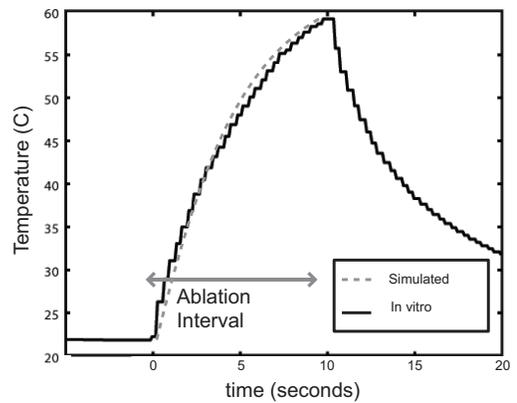
Fig. 3. Temperature rise in a piece of tissue measured by a type E micro-thermocouple. A 10W, 10MHz CW, 10 second signal was applied to the transducer in our fixed focus setup (Fig.2). A temperature rise of 45°C was observed.
