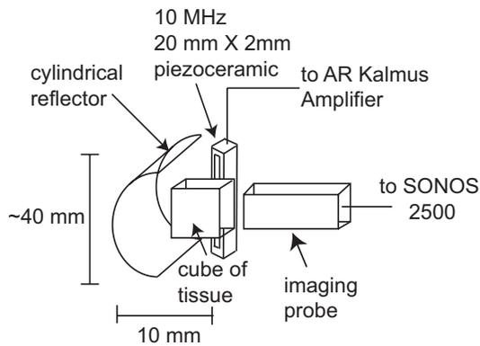
Fig. 2. A 10 MHz, 20 mm by 2 mm transducer was used for fixed focus ablation, with a focusing cylindrical mirror (focal length of 10 mm). The transducer was angled to produce an off-axis lesion in a piece of tissue. Running water was pumped over the tissue to simulate convection from blood. A 0.25 mm diameter micro-thermocouple was placed inside the tissue to measure the temperature rise at the focal point. The lesion was imaged using a 5 MHz SONOS 2500 ultrasound probe.
