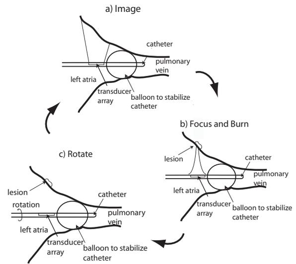
Fig. 1. An illustration of the catheter function. (a) The array will image the region of interest. (b) The anatomy and location of previously formed lesions will be identified and used to dynamically focus the therapy. (c) The catheter will be rotated and the process will repeat until a contiguous circumferential lesion is formed around the pulmonary vein.
