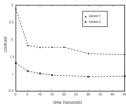
Fig. 7. The contrast of the lesions over time as measured by averaging the lesion brightness and then dividing by the brightness of the same area in the pre-HIFU image. The decay seems to be exponential with time constant between 5-10 seconds. One lesions seemed to have a contrast twice as large as the other lesions; during the formation of lesion, we observed what appeared to be mechanical motion in the lesion area indicating possible mechanical effects.
