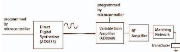
Fig. 8. Diagram of one channel of the ablation electronics system. A microcontroller programs frequency and phase of the DDS and gain stage. The output signals are then amplified and applied to the transducer elements.
