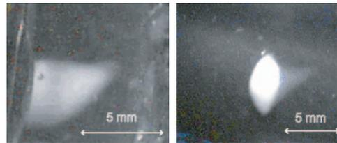
Fig. 4. Pictures of a HIFU lesion formed by our fixed focus system (Fig. 2) in the focal plane (right) and along the direction of propagation (left) formed in a HIFU gel that changes from clear to opaque at 55°C.
