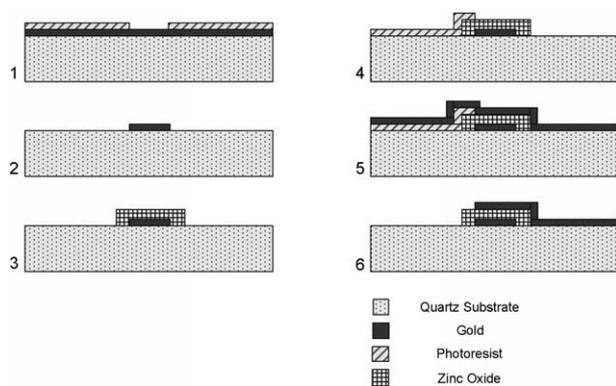
Fig. 2. Fabrication steps for the PZT element.
