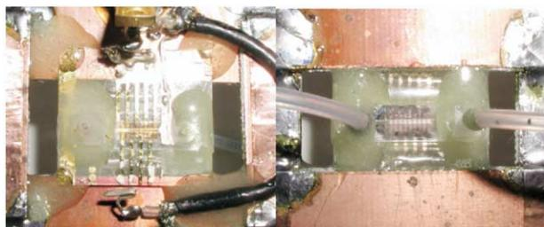
Fig. 3. Microfluidic device with integrated transducers. (a) Channel side, and (b) transducer side.
