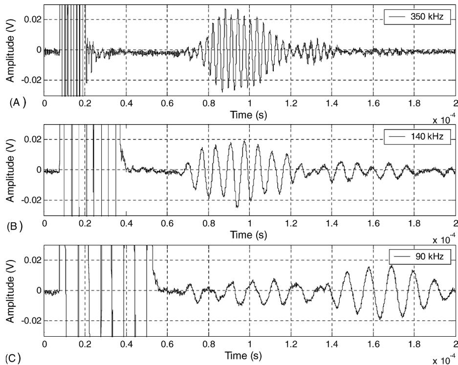
Fig. 11. Three received signals with a 4 sine wave cycle excitation at different frequency (A) 350 kHz, (B) 140 kHz, (C) 90 kHz.
