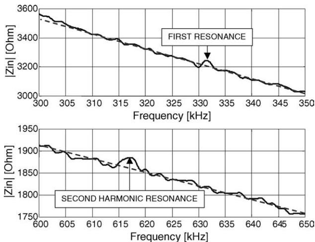
Fig. 9. Measured input impedance of the embedded interdigital transducer.
