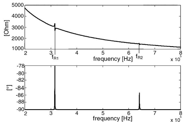
Fig. 7. Simulated electrical impedance  $Z_{\text{IN}}$  of the embedded interdigital transducer: magnitude (top) and phase (bottom).
