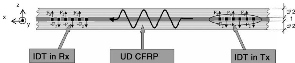
Fig. 4. Schematic drawing of an IDT pairs embedded in a unidirectional CFRP sample. The reference axis of the experiment is shown and the the polarization axis '1', '2', '3' of the piezo-polymer film.
