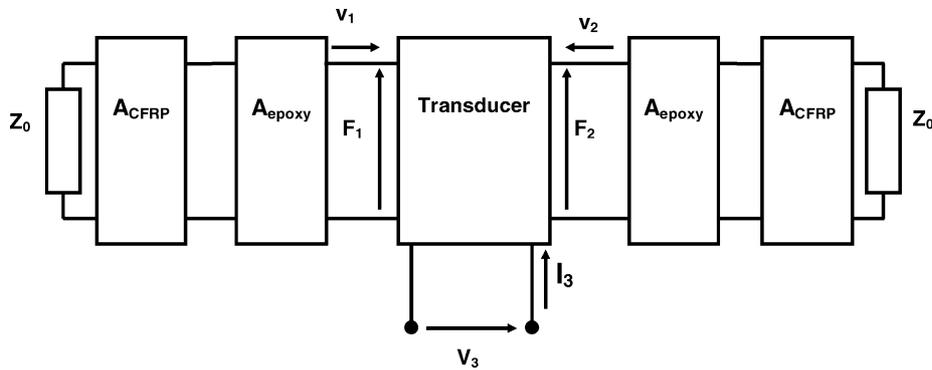
Fig. 5. Equivalent three-port model for piezoelectric interdigital transducer. Parameters description for layers 1 and 2:  $F_i$ : force (N)  $i=1, 2$ ;  $v_i$ : longitudinal velocity (m/s)  $i=1, 2$ ;  $V_3$ : voltage (V);  $I_3$ : current (A);  $A_{\text{epoxy}}$ : acoustic transmission line matrix of the epoxy glue layer;  $A_{\text{CFRP}}$ : acoustic transmission line matrix of the unidirectional CFRP layer;  $Z_0$ : characteristic impedance of the semi-infinite medium (air in our case).
