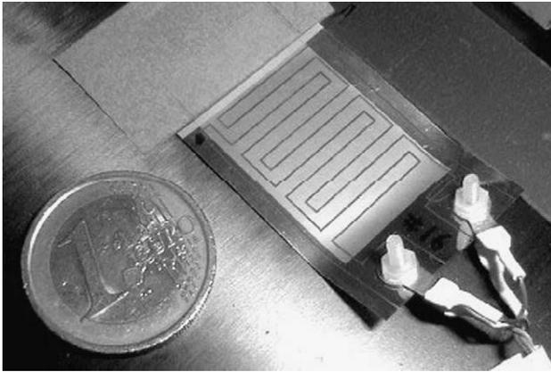
Fig. 3. Prototype of the interdigital piezopolymer transducer bonded on a unidirectional 1.5 mm thick unidirectional CFRP laminate before the application of the epoxy.
