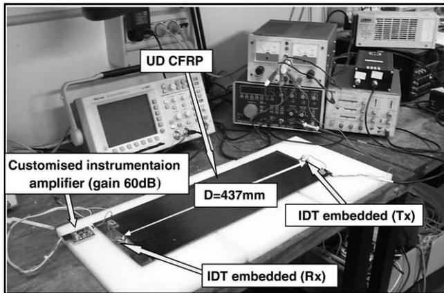
Fig. 8. Experimental set-up used to validate the design process.
