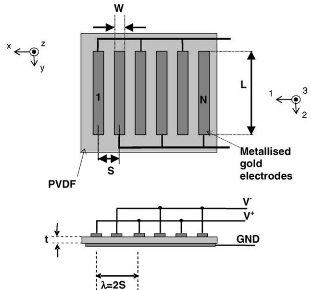
Fig. 1. Configuration of an IDT bonded on a laminate. (Top) plane view, (bottom) cross-section view. Drawing not in scale.
