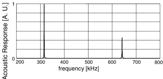
Fig. 6. Simulated acoustic response of interdigital transducer.
