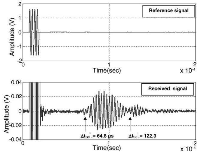
Fig. 10. Burst of four sinusoidal cycles at  $f_0 = 350$  kHz used as reference signal (top) and received signal on the Rx-IDT (bottom). The predicted values of time of flight for the two propagation modes are indicated as  $\Delta t_{SO}'$  and  $\Delta t_{SO}''$ .
