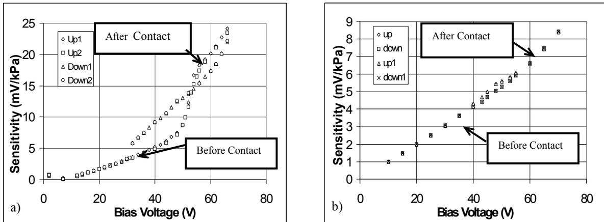
Figure 2. Ultrasonic reception by CMUT as a function of bias voltage. Source: a PZT transducer with a constant output. a) Conventional CMUT: hysteresis is evident after membrane-bottom electrode contact (collapsed region operation). b) PostCMUT: good repeatability and no hysteresis after membrane-post contact.
