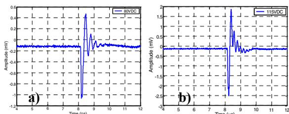
Figure 4. Transmission pulses obtained by a hydrophone from a PostCMUT operating a) before contact and b) after contact. The input AC signal was a 5V step function.
