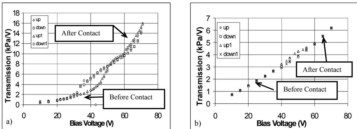
Figure 3. Ultrasonic transmission by CMUT received by a broad band hydrophone as a function of bias voltage. a) Conventional CMUT: hysteresis is evident after membrane-bottom electrode contact (collapsed region operation). b) PostCMUT: good repeatability, normal looking curve shape and no hysteresis after membrane-post contact.
