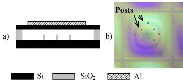
Figure 1. a) Cross-sectional view of a PostCMUT. b) Photograph of fabricated devices with 9-point post patterns.
