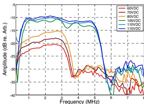
Figure 5. Transmission spectrum (uncorrected) of a PostCMUT at different bias voltages.
