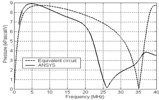
Figure 8. Transmit pressure calculated on the transducer's surface.
