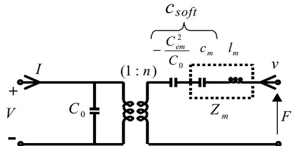
Figure 1. Electrical equivalent circuit of a CMUT.
