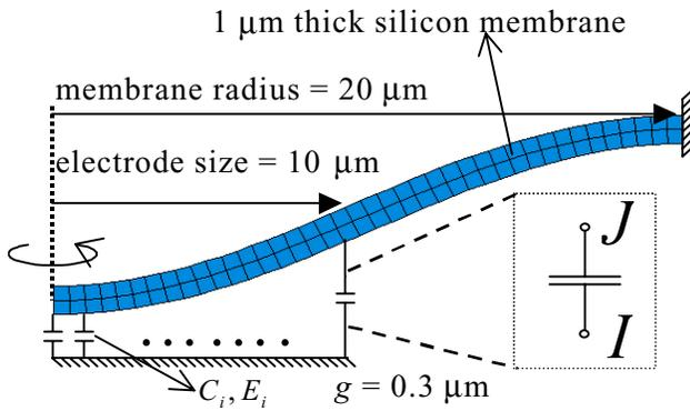
Figure 2. Finite element model for vacuum calculations
