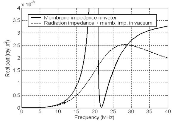
Figure 6. Real part of the membrane impedance calculated using equivalent circuit approach and FEM.
