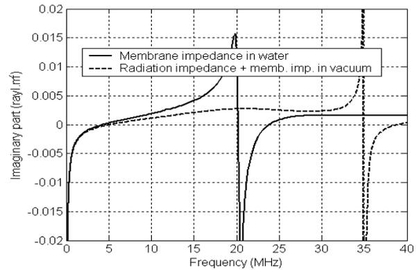
Figure 7. Imaginary part of the membrane impedance calculated using equivalent circuit approach and FEM.
