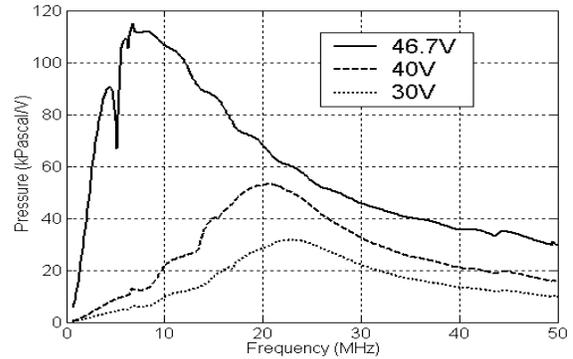
Figure 10. Transmit pressure of a 1D array.
