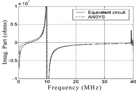
Figure 4. Input impedance using improved circuit model and FEM.
