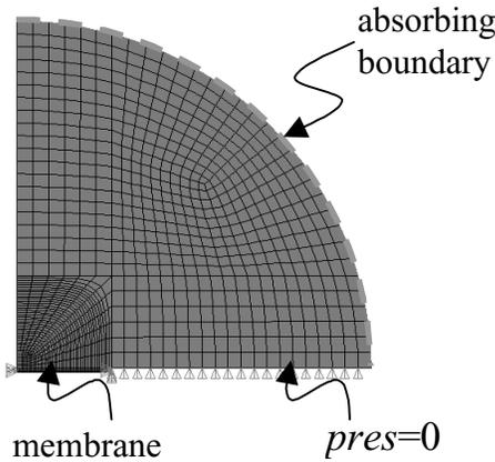
Figure 5. FEM mesh for a single membrane.
