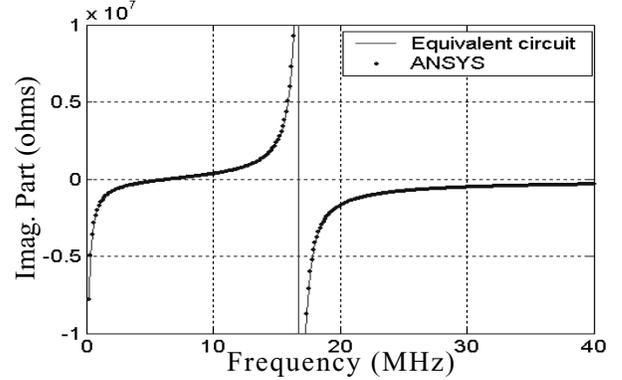
Figure 3. Input impedance for a parallel plate capacitor.
