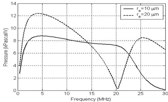
Figure 6. Transmit pressure. The pressure is calculated  $\lambda$  away from the transducer surface.
