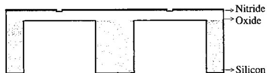
Patterning 5 microns orifices in the nitride by dry etch
