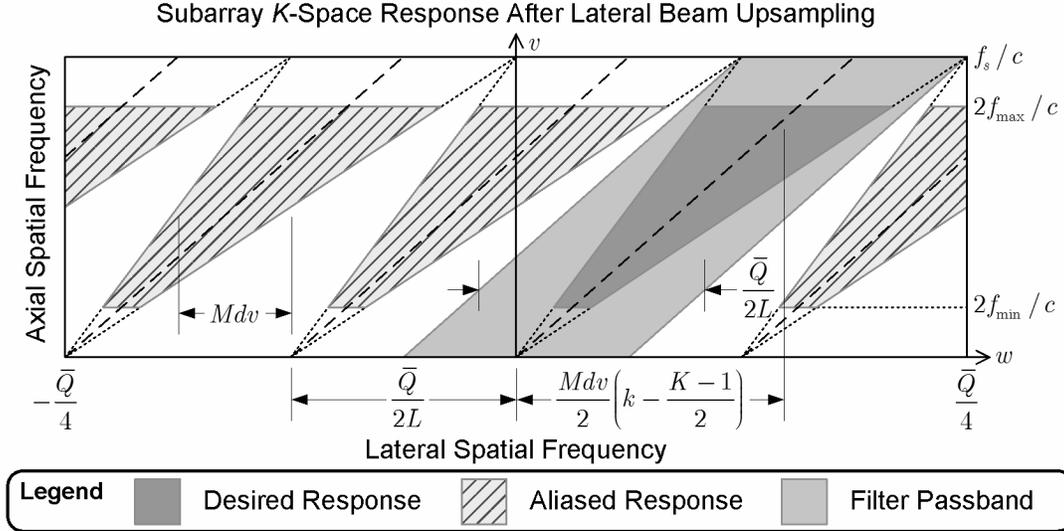
**Figure 1.** Spatial frequency response of a single subarray after beam upsampling and before reconstruction filtering. The dimensions are given for the general case; the passband regions shown correspond to an off-center subarray and an upsampling rate of  $L=4$ .
