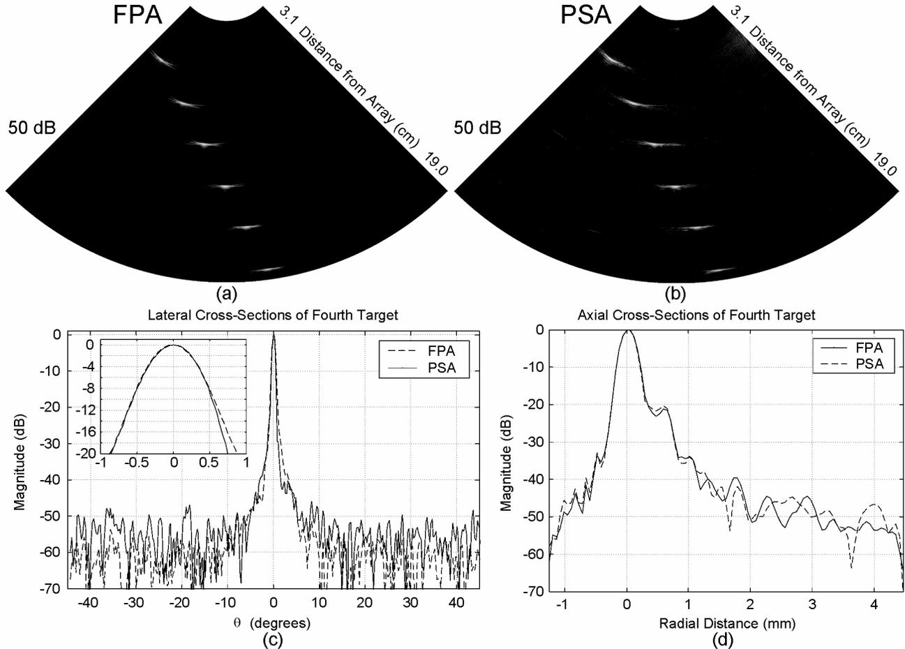
**Figure 2.** Comparison of experimental wire target images formed by conventional FPA imaging and PSA imaging using wideband reconstruction filters. A 128-element CMUT array was used. The PSA configuration consisted of 32 front-end channels, reducing the front-end hardware complexity by a factor of 4.
