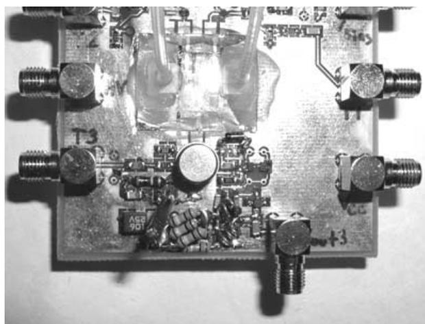
Figure 1. Picture of a printed circuit showing the assembled micro-channel and transducer along with the necessary electronics
