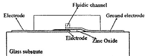
Figure 2. The cross-section of a piezoelectric transducer
