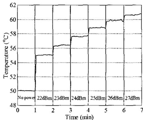
Figure 8. Temperature measurements by varying power applied for heating
