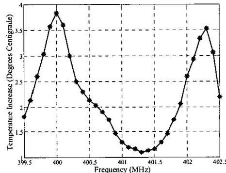
Figure 7. Variation of heating with frequency of applied tone bursts
