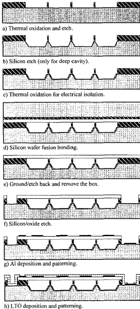
Fig. 1: Major steps of CMUT fabrication using wafer-bonding technique.
