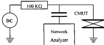
Fig. 4: Experimental setup used for measuring the electrical input impedance of the CMUT.
