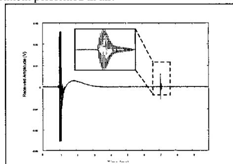
Fig. 6: The pulse-echo experiment result of a low frequency CMUT in the air. The enlarged window shows the reflected pulse. The reflector is a steel block 1meter from the transducer.
