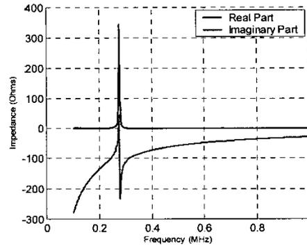
Fig. 5 Electrical input impedance of the CMUT as measured by the vector network analyzer.
