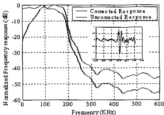
Fig. 7: The uncorrected spectrum (red) and the spectrum corrected for attenuation and diffraction (blue) of the pulse in oil
