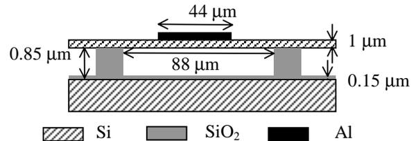
Figure. 1. The cMUT simulation used in the simulations.
