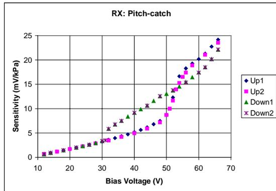
Figure 6. The receive sensitivity of the cMUT element as a function of bias.
