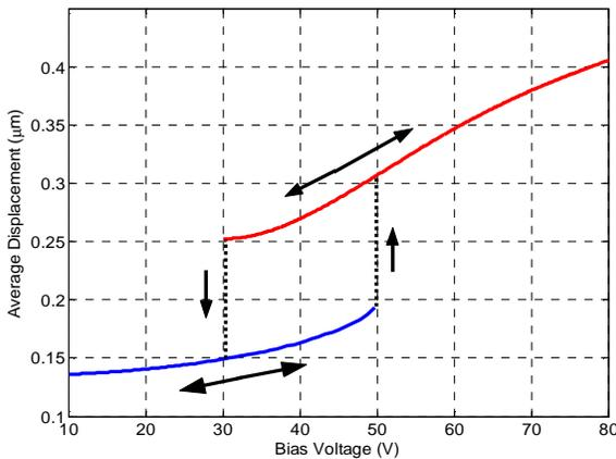
Figure 3. The simulated static membrane displacement .
