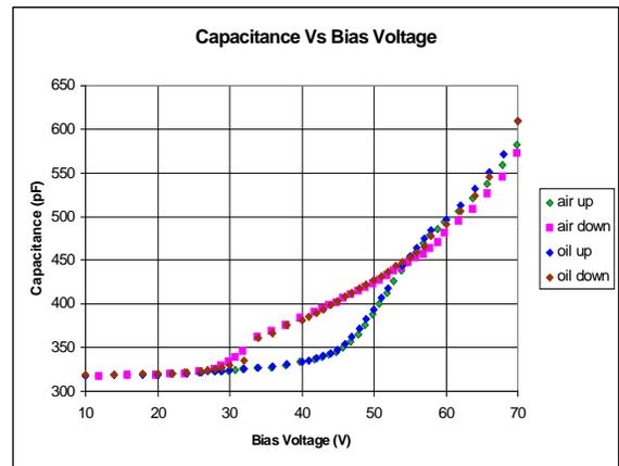
Figure 4. The capacitance of the cMUT element as a function of bias, measured.
