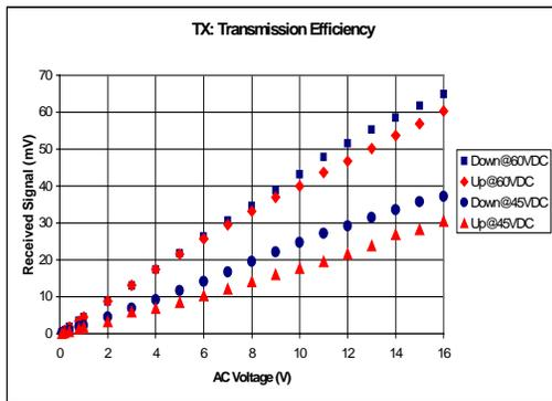
Figure 8. The signal transmitted by the cMUT element as a function of applied AC signal.
