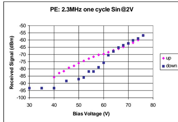
Figure 7. The pulse echo signal received by the cMUT element as a function of bias.
