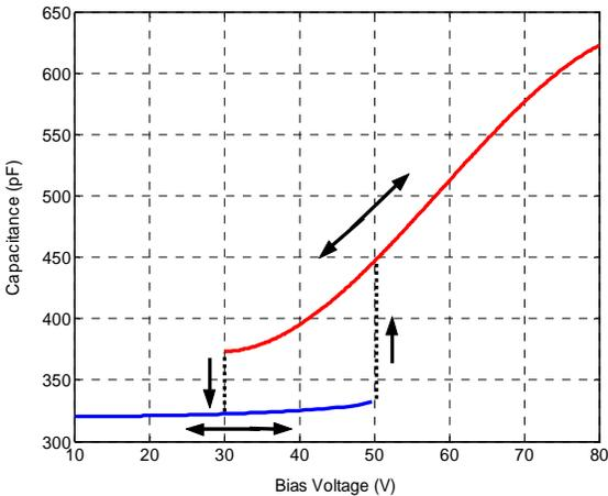
Figure 2. The simulated capacitance of the cMUT element as a function of bias.
