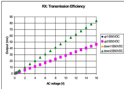
Figure 9. The signal received by the cMUT as a function of AC signal applied to a PZT transmitter.
