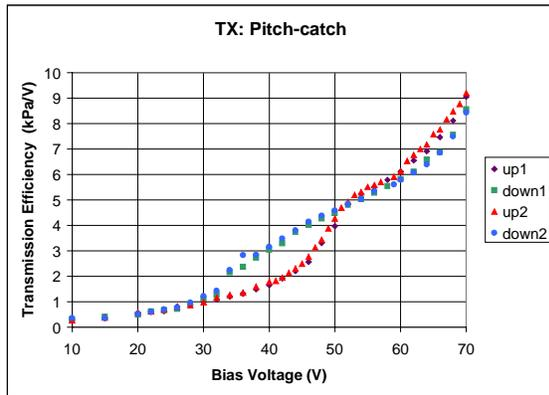
Figure 5. The transmission efficiency of the cMUT element as a function of bias.
