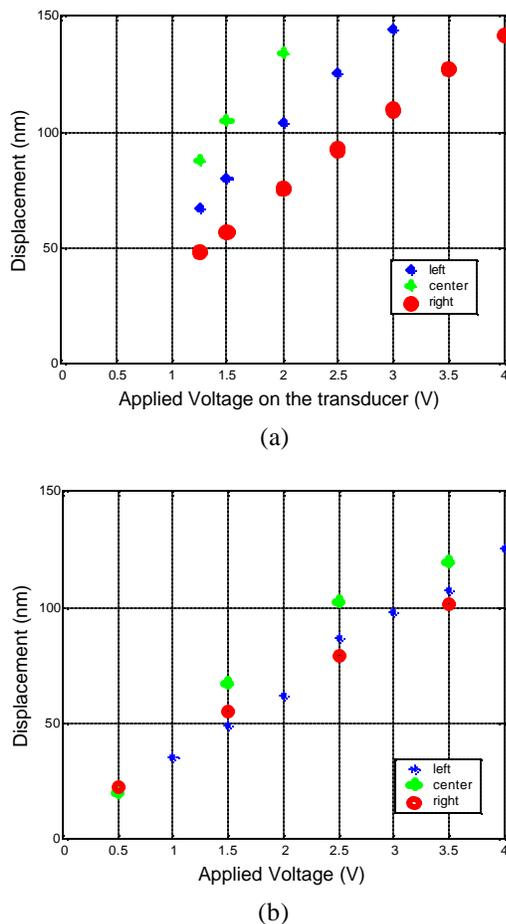
Figure 7. Maximum displacements on three membrane centers across the array (a) with 500 μm reservoirs (b) no reservoirs.
