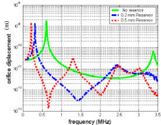
Figure 2. 3D FEM results: Maximum orifice displacement of a single membrane vs. frequency of an ejector array of  $160 \mu\text{m}$  in diameter  $\text{Si}_x\text{N}_y$  membranes with and without reservoir.
