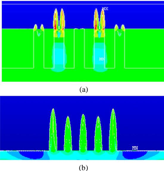
Figure 4. Orifice displacement of array membranes at resonance (a) with a  $500\ \mu\text{m}$  reservoir (b) without an individual reservoir (not to scale).
