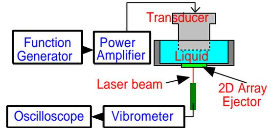
Figure 6. Experimental setup.
