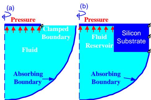
Figure 1. Unit Cell of an ejector array for 3D FEM simulations: (a) No Reservoir, (b) With reservoirs.
