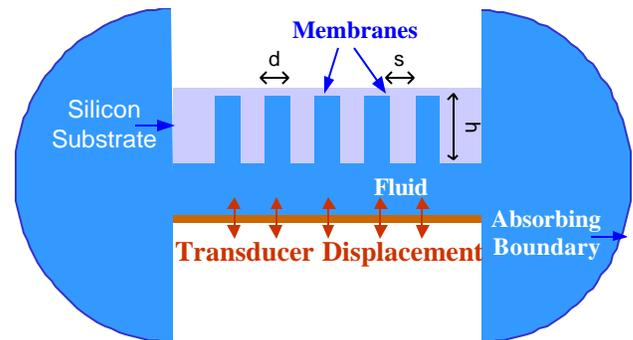
Figure 3. FEM model of  $1 \times 5$  ejector array with transducer.
