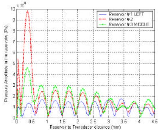
Figure 5. Pressure amplitude along a line across three reservoirs of the ejector array during actuation.
