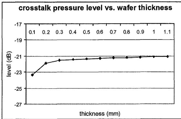
(a) change of wafer thickness
