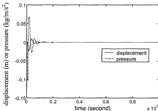
Fig. 3. Transient responses of the receiver cMUT,  $R_1$ , in Fig. 1.
