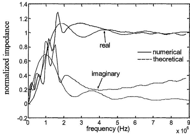
Fig. 7. Radiation impedance  $z$  of a cMUT array.
