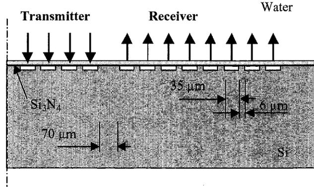
Fig. 6. Schematic view of an underwater cMUT array transducer.
