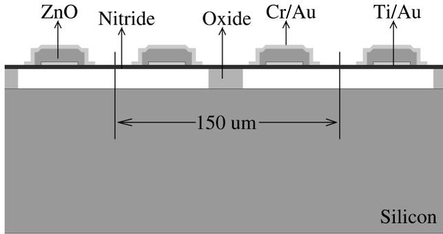
Fig. 1. Side view of two adjacent cells of the developed micromachined two-dimensional array of transducers.
