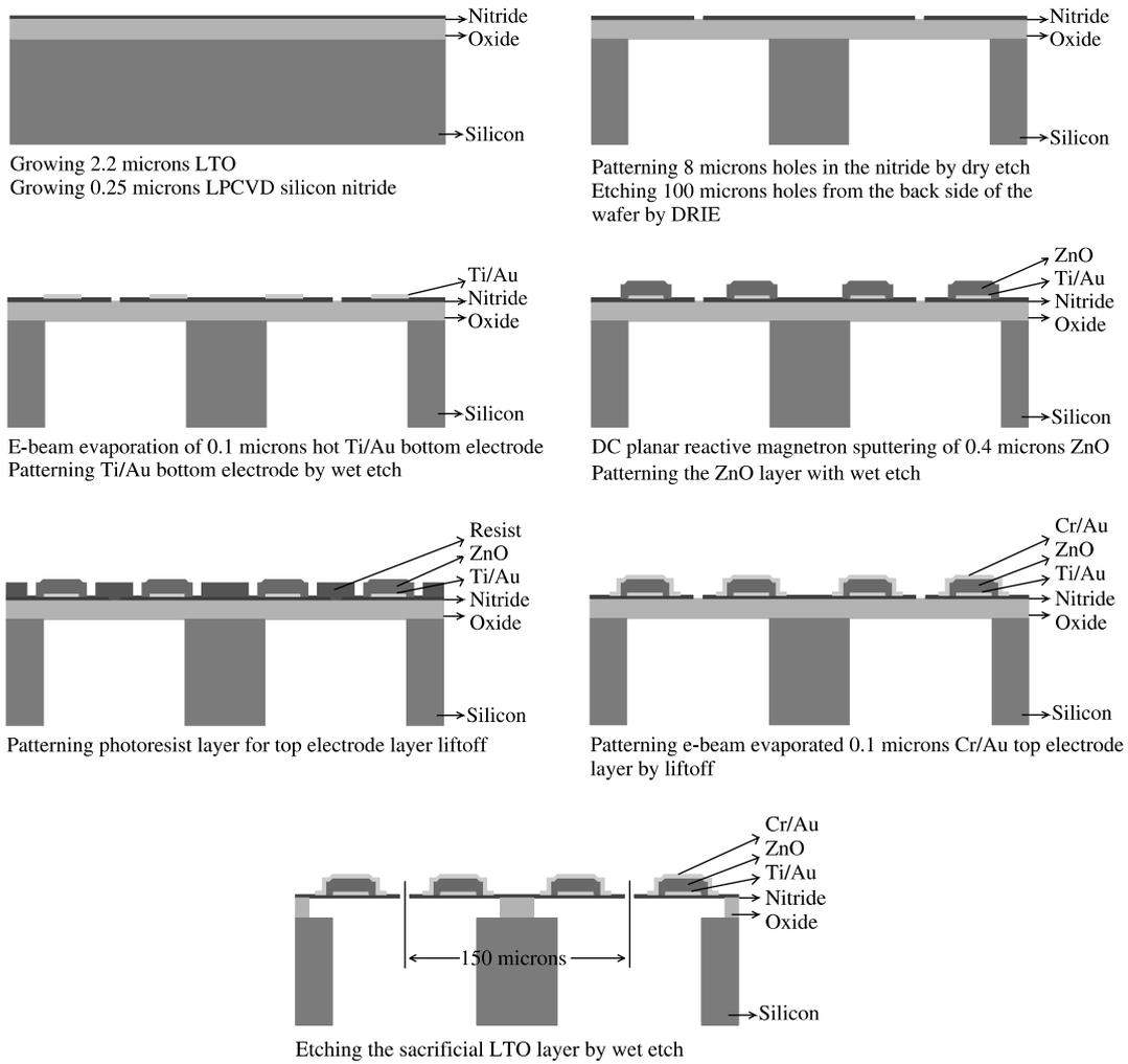
Fig. 7. The second micromachined device process flow.
