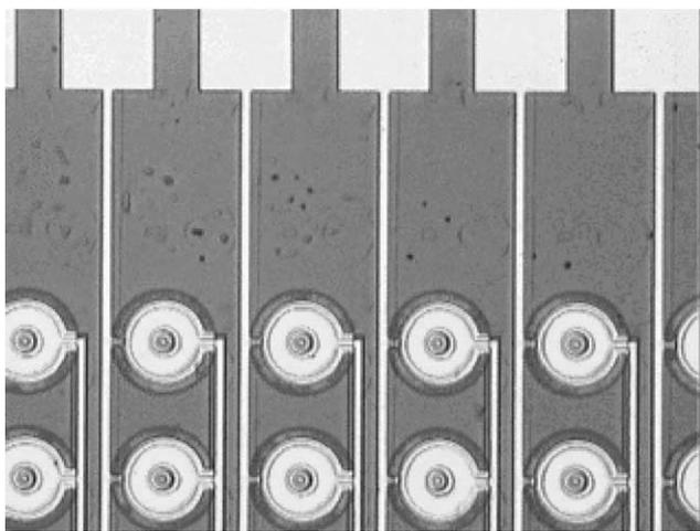
Fig. 8. Realized micromachined device: individual cells are 100  $\mu\text{m}$  in diameter.
