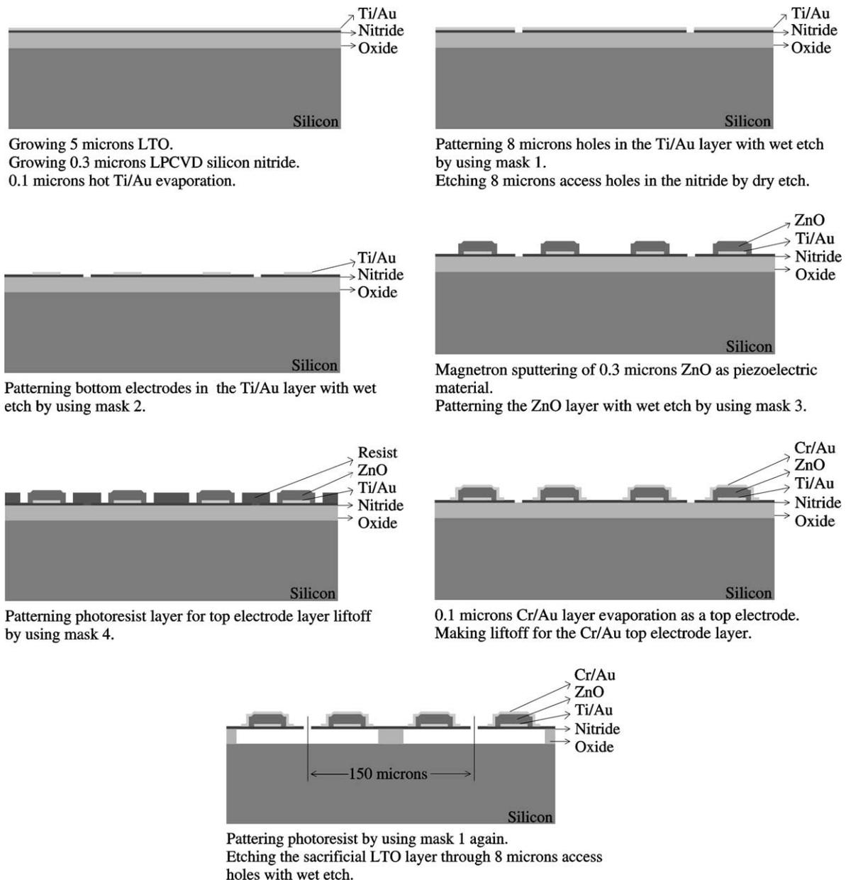
Fig. 6. First micromachined device process flow.
