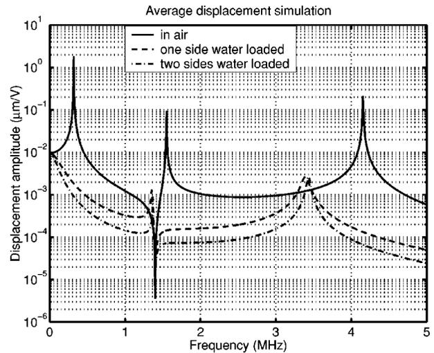
FIG. 2. Micromachined droplet ejector average displacement simulations for a single element for air and water loaded cases.
