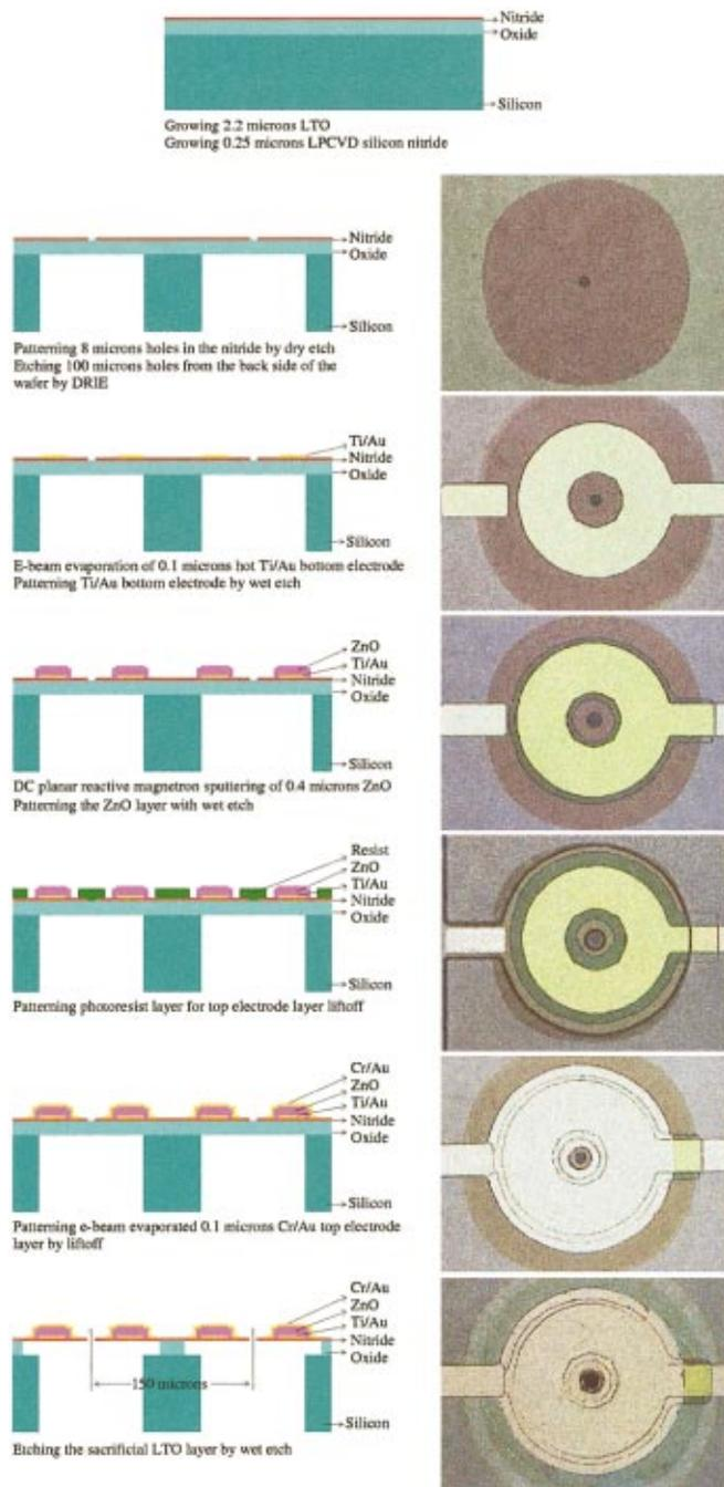
FIG. 3. (Color) Micromachined droplet ejector fabrication process flow.
