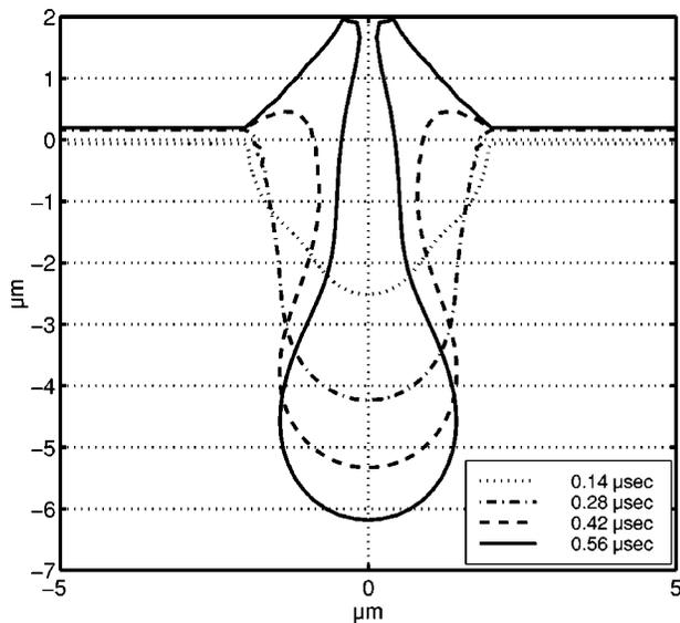
FIG. 1. Typical microelectromechanical systems device water ejection simulation through 4  $\mu\text{m}$  diameter orifice at 1.4 MHz by using 112  $\mu\text{m}$  diameter device. The drop formation is shown at different time intervals.
