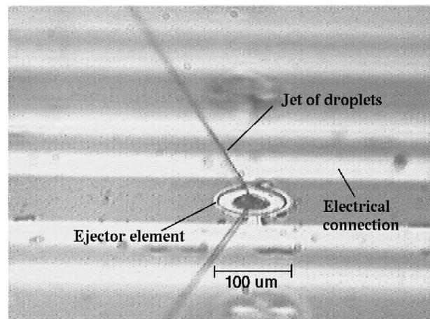
FIG. 5. Water ejection through 5  $\mu\text{m}$  diameter orifice at 3.48 MHz by using both the first and the second type of operation.
