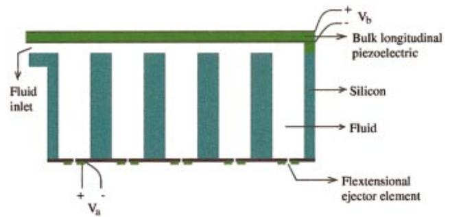
FIG. 4. (Color) Configuration of the micromachined droplet ejector. The device is bulk actuated by using the bulk piezoelectric material.
