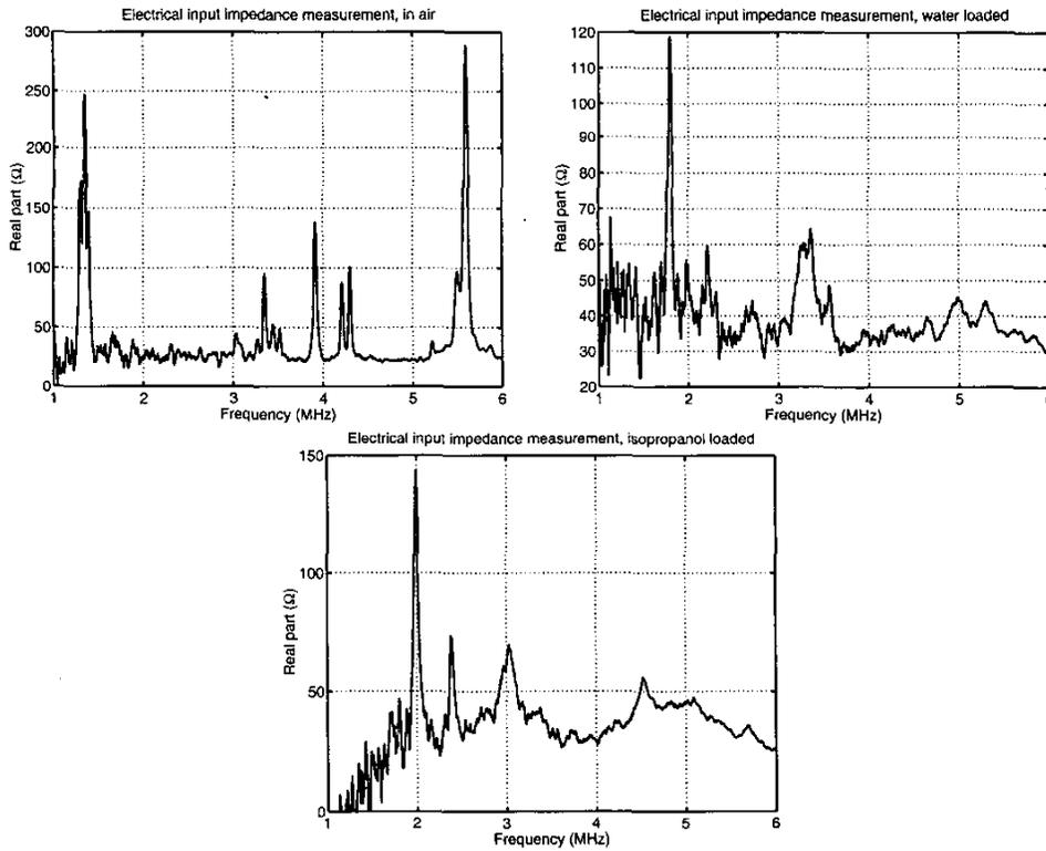
Fig. 15. Type II micromachined flextensional transducer measurements (Device E; four elements are connected).
