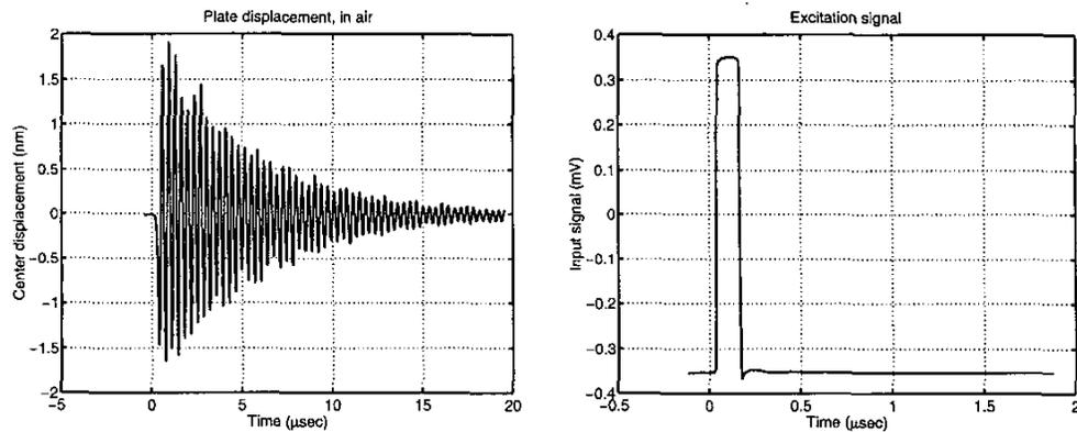
Fig. 9. Type I micromachined flextensional transducer interferometer measurements (Device B).
