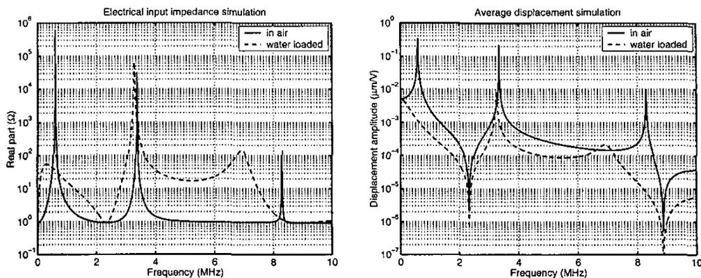
Fig. 2. Type I micromachined flextensional transducer simulations for a single element (Devices A, B, and C).
