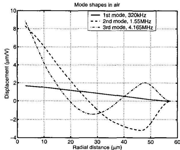
Fig. 17. Type II micromachined flexensional transducer simulations for a single element (Device E).
