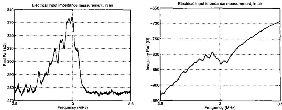
Fig. 10. Type I micromachined flextensional transducer measurements (Device B; 60 elements are connected).
