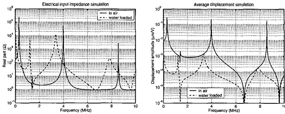
Fig. 12. Type II micromachined flextensional transducer simulations for a single element (Device D).
