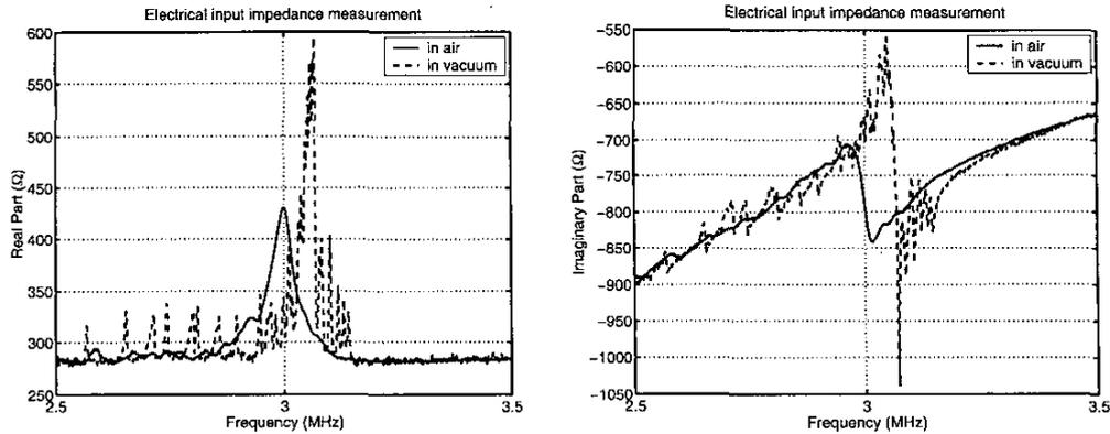
Fig. 1. Type I micromachined flextensional transducer measurements (Device A; 60 elements are connected).
