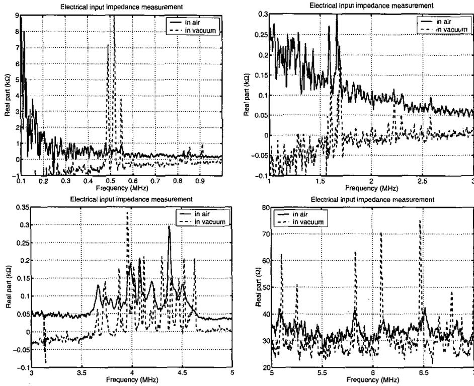
Fig. 11. Type II micromachined flextensional transducer measurements (Device D; three elements are connected).
