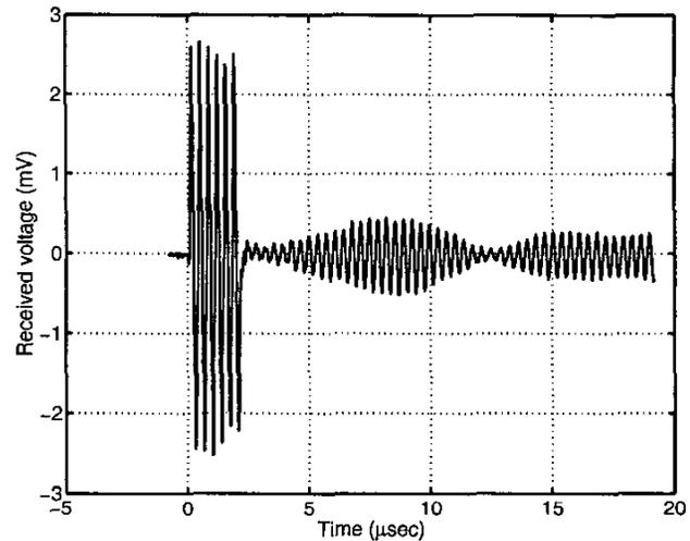
Fig. 7. Type I micromachined flextensional transducer air transmit/receive measurements (Devices A and C).
