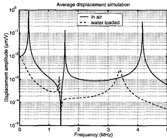
Fig. 16. Type II micromachined flexensional transducer simulations for a single element (Device E).
