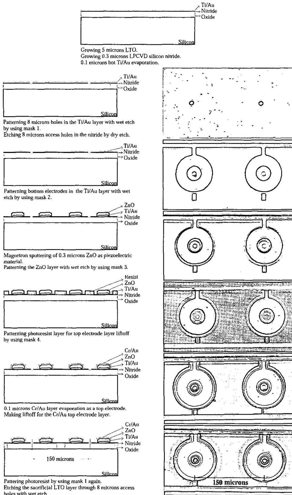
Fig. 3. Realized Type I micromachined device fabrication process flow.
