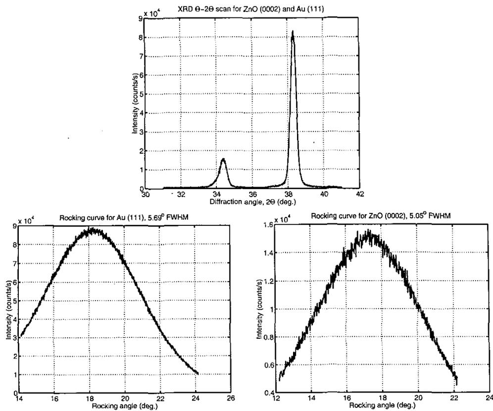
Fig. 4. X-ray diffraction measurements of ZnO (0002) and Au (111) films.
