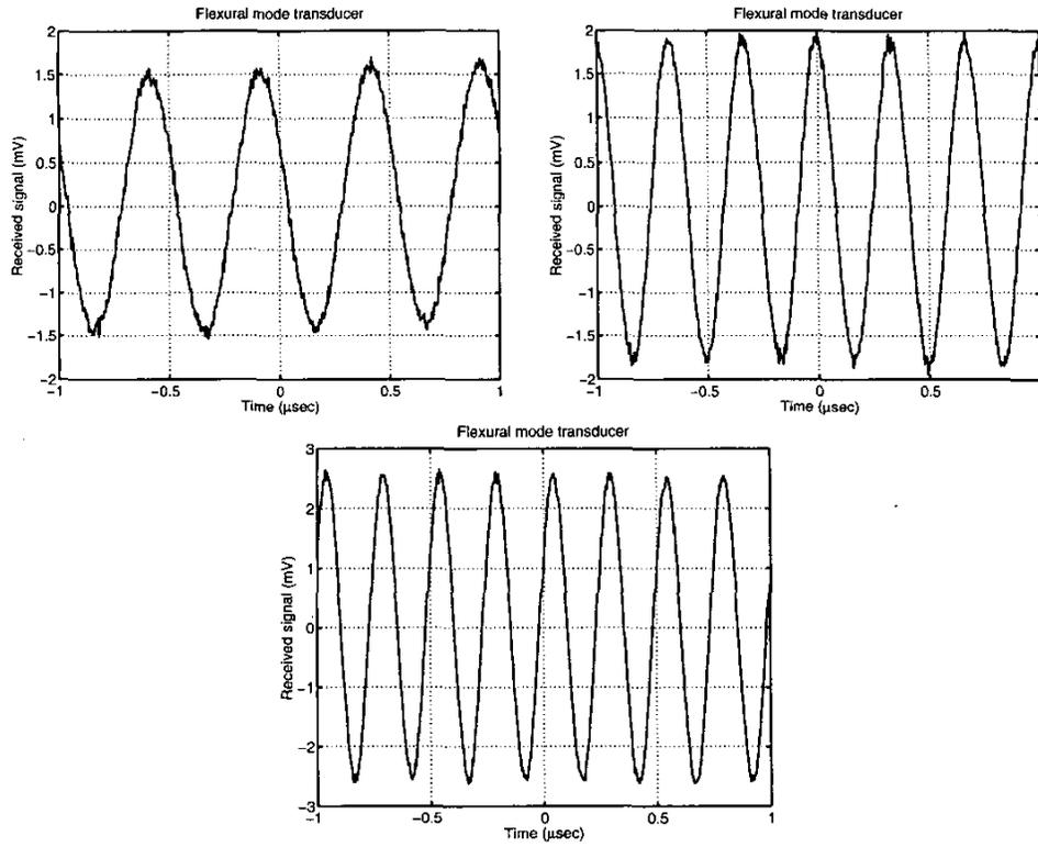
Fig. 14. Water-loaded Type II micromachined flextensional transducer measurements (Device E; four elements are connected).
