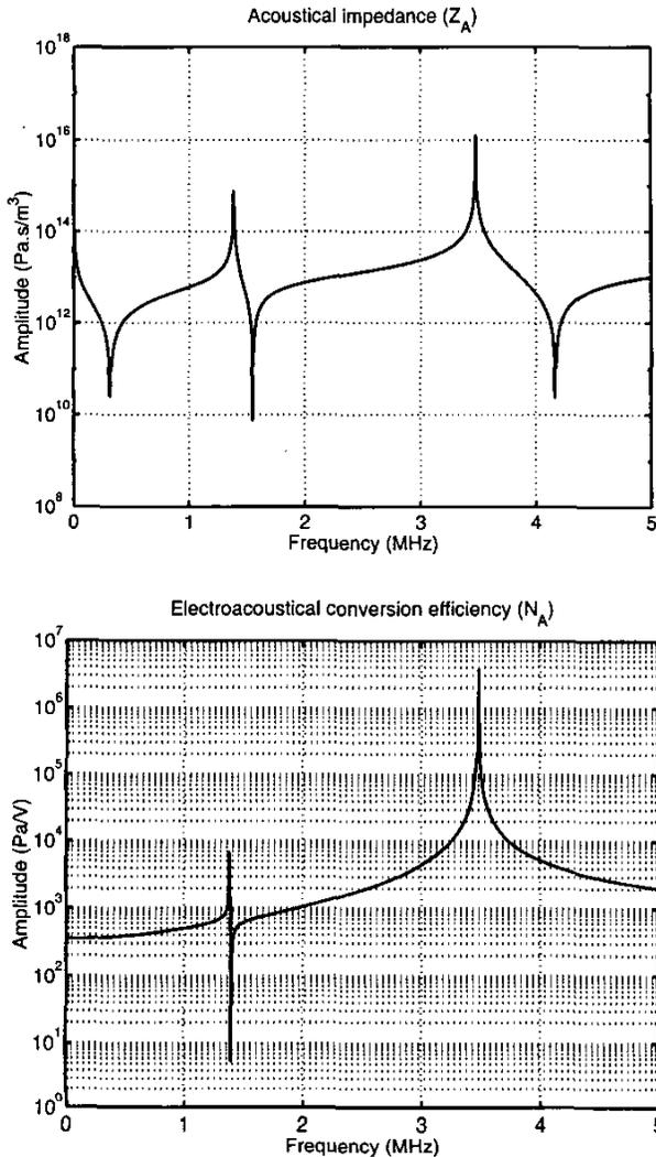
Fig. 18. Type II micromachined flextensional transducer simulations for a single element (Device E).
