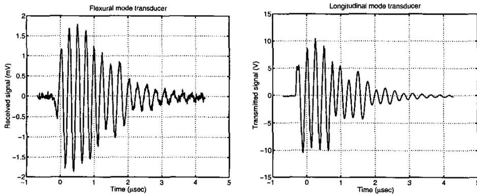
Fig. 13. Water-loaded Type II micromachined flextensional transducer measurements (Device E; four elements are connected).
