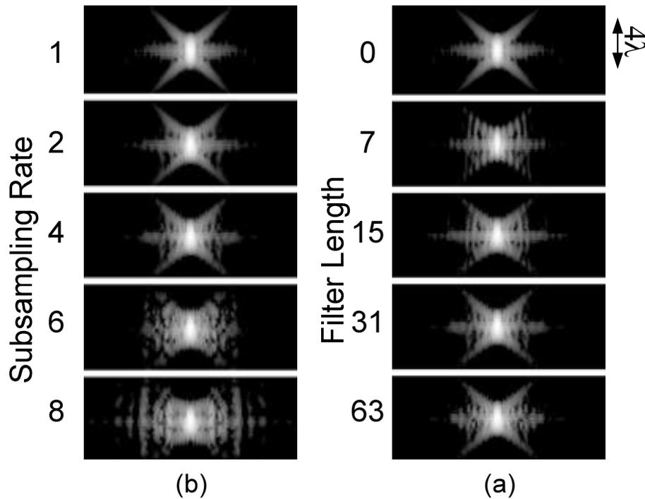
**Figure 9.** (a) PSF dependence on subsampling rate. The filter length varies such that each beam is reconstructed using four acquired beams. (b) PSF dependence filter length. A subsampling rate of 4 is used, and filters of varying lengths are used to reconstruct the PSFs. All PSFs shown were formed using MSA-M, but MSA-P and MSA-F are equivalent and have imperceptible differences.
