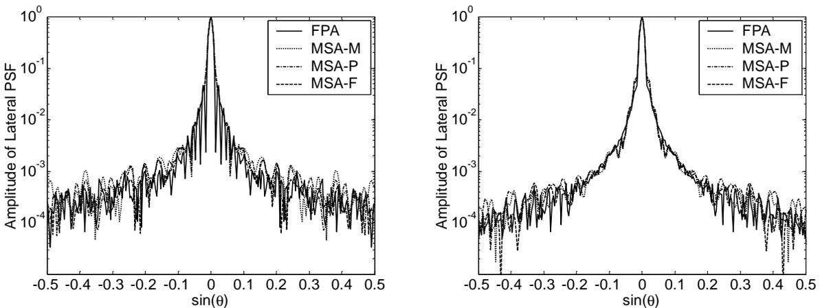
**Figure 7.** 1D lateral PSFs for 10% and 50% bandwidth. The 3 dB lateral resolution for all image reconstruction methods is  $0.90^\circ$ .
