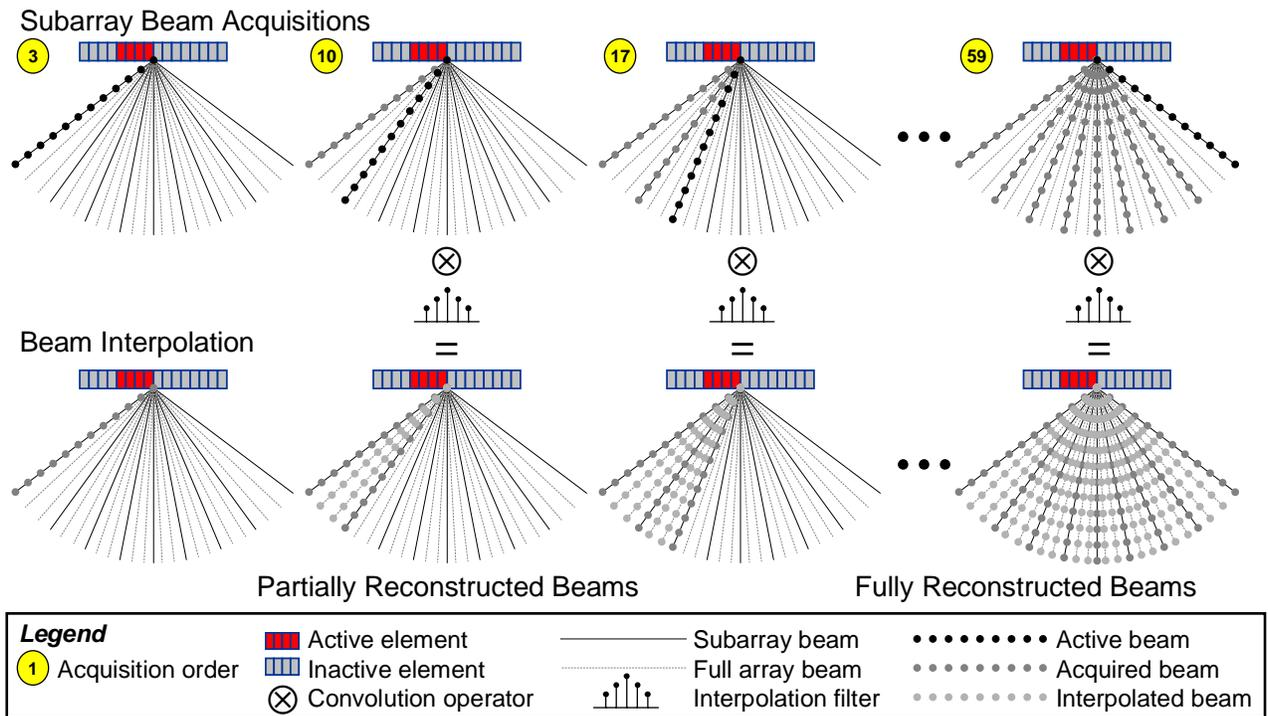
**Figure 4.** Beam interpolation. As the low beamrate beams are being acquired, interpolation filters reconstruct the remaining beams which will form the high beamrate image.
