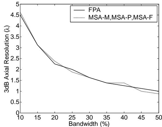
**Figure 8.** 3 dB axial resolution dependence on signal bandwidth. As expected, wider bandwidth pulses correspond to lower axial resolutions. The resolution obtained from all MSA methods closely approximates that of conventional FPA imaging.
