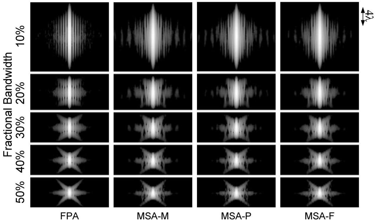
**Figure 6.** 2D PSF results at varying signal bandwidths. Simulation results showing the how the pulse bandwidth affects the PSF. The responses of all MSA imaging methods have imperceptible differences. Their responses can be compared to the best PSF obtained by from using FPA imaging. Each PSF is  $30^\circ$  wide, evenly spaced in  $\sin\theta$ , and displayed with 60 dB of logarithmic compression.
