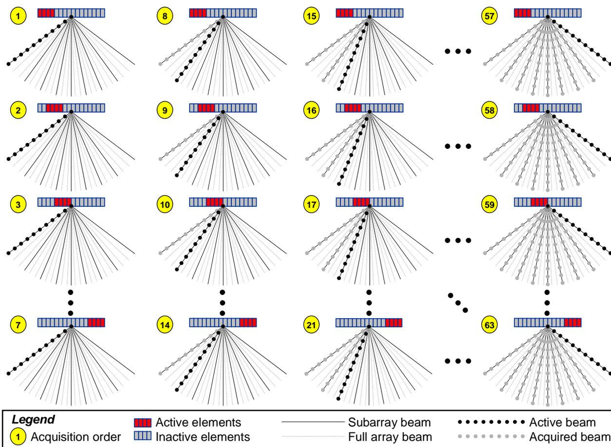
**Figure 3.** Subarray beam acquisition steps. Each subarray is used to acquire a subset of the beams that would normally be acquired for FPA imaging. This subset of beams forms a low beamrate image. All subarrays sample the same beam sequentially in order to reduce motion artifacts.
