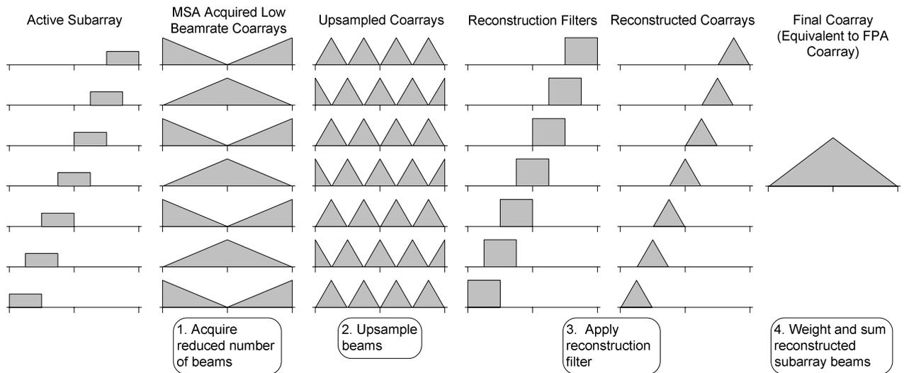
**Figure 1.** Coarray responses at each stage of the multi-element synthetic aperture (MSA) image formation algorithm. Ideally, the reconstructed coarrays will equal the coarray that would be obtained from each subarray if full beamrate samples were acquired. The resulting coarray is equivalent to that of the FPA imaging method.
