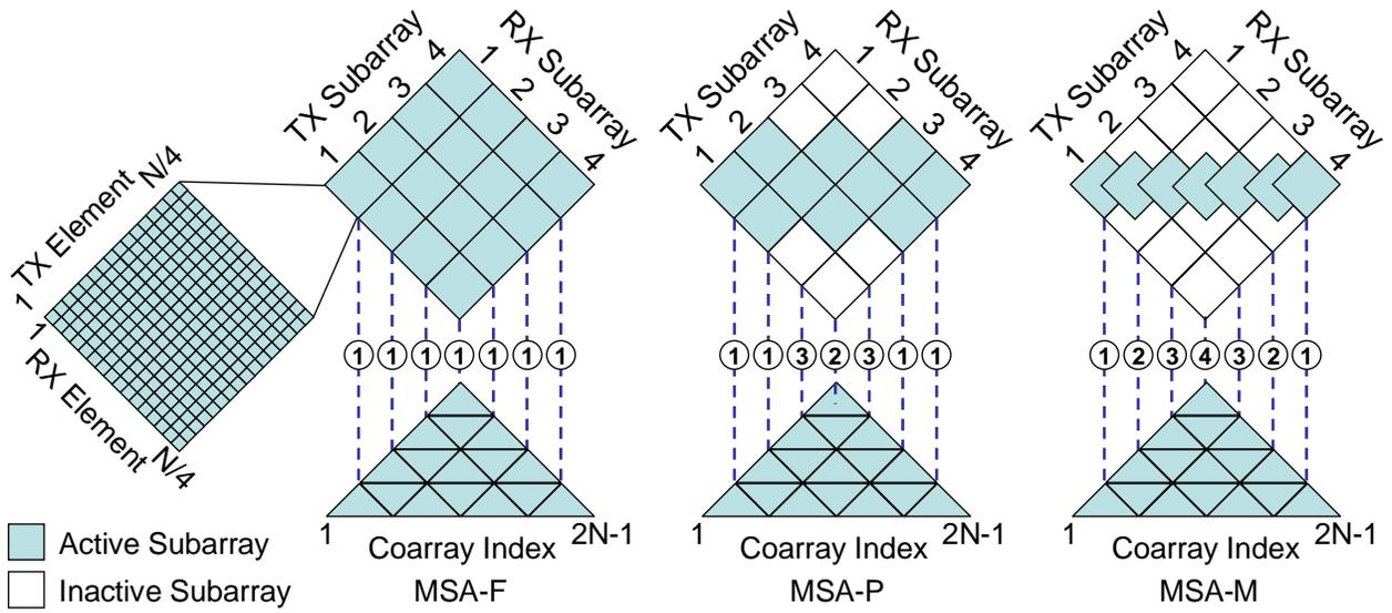
**Figure 2.** Coarray representation of three different multi-element synthetic aperture image reconstruction methods. Each TX and RX subarray combination contributes to different lateral spatial frequencies represented by the coarray. Weighting and summing of the subarray responses approximates the coarray of conventional full-phased array (FPA) imaging.
