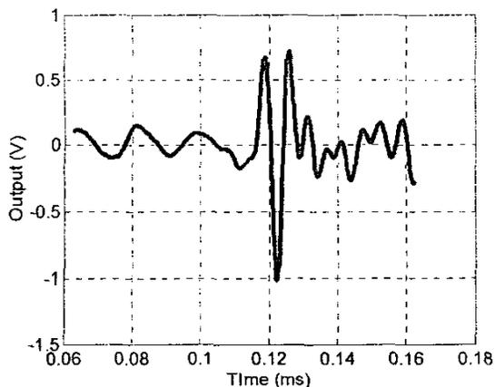
Fig. 7: Impulse Response of the CMUT transducer.
