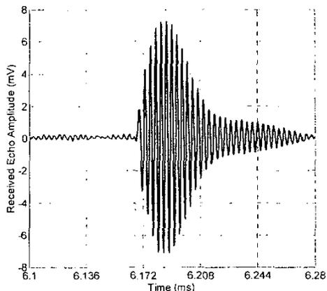
Fig. 6: The result of the pulse echo experiment in air, showing a narrow frequency band operation.
