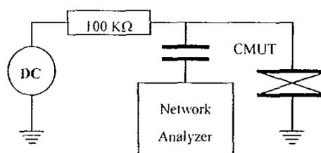
Fig. 4: Experimental setup used for measuring the electrical input impedance of the CMUT.
