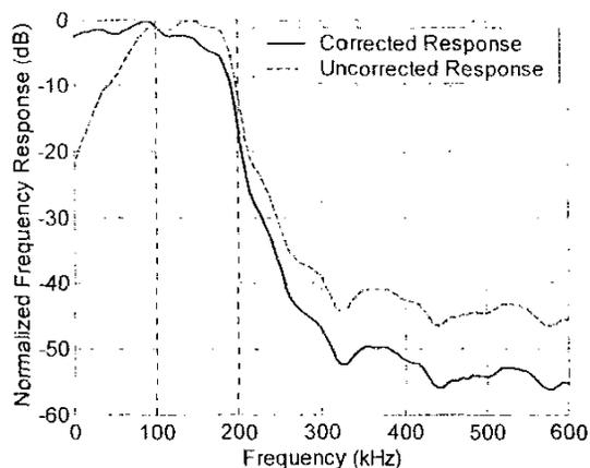
Fig. 8: The uncorrected spectrum (red) and the spectrum corrected for attenuation and diffraction (blue) of the pulse in Fig. 7.
