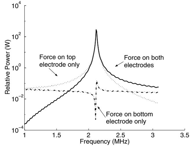
Fig. 4. Power coupled into the  $A_0$  mode of the substrate using three different excitation mechanisms. The constants are taken from Auld:  $V_s = 5840.9$  m/s,  $V_l = 8429.4$  m/s,  $\rho = 2332$  kg/m<sup>3</sup>.
