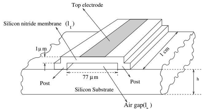
Fig. 1. Diagram of a single CMUT membrane.
