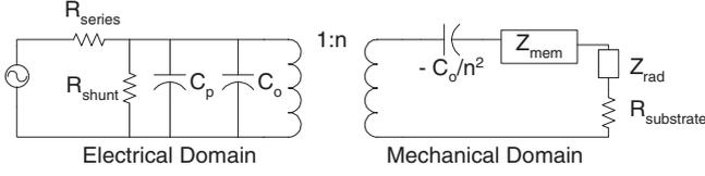
Fig. 2. Equivalent circuit model of a transmitting CMUT.
