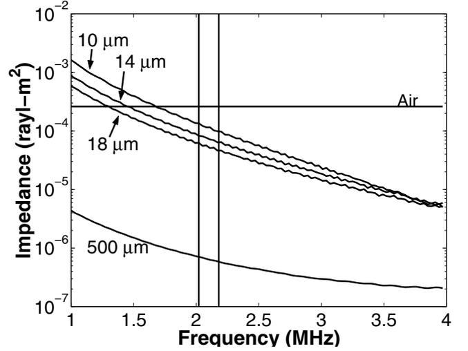
Fig. 3. Impedance presented to the vibrating membrane by device substrates of four different thicknesses. The vertical lines represent the operating frequency range of the four devices.
