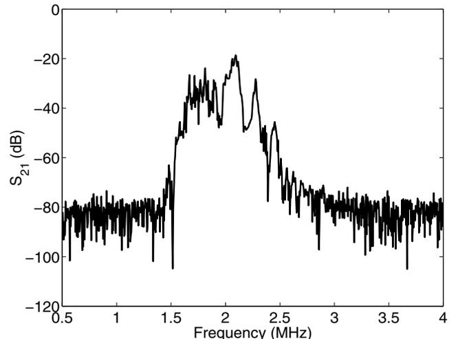
Fig. 6. An  $S_{21}$  measurement of a Lamb wave device. Note that the insertion loss near 2.1 MHz is 20 dB.
