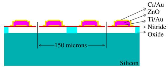
Patterning photoresist by using mask 1 again.
