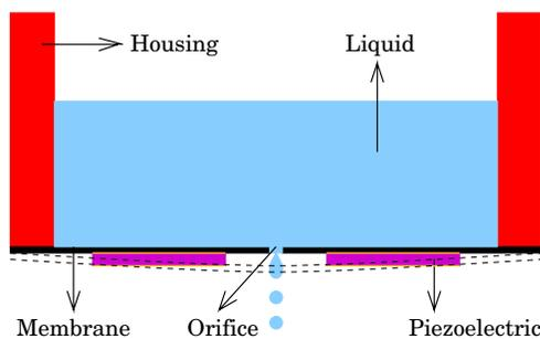
Figure 2: A schematic of the large-scale prototype ejector: the lateral extent is 9 mm
