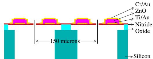
Etching the sacrificial LTO layer by wet etch
