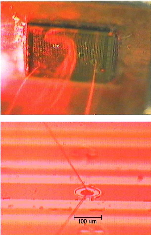
Figure 7: Water ejection by using a micromachined fluid ejector, 3.5 millions 4 μm diameter water droplets per second are ejected
