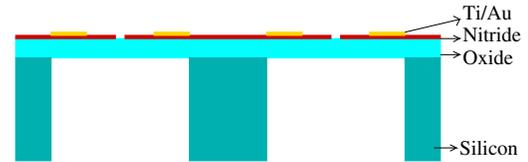
E-beam evaporation of 0.1 microns hot Ti/Au bottom electrode
