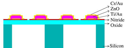
Patterning e-beam evaporated 0.1 microns Cr/Au top electrode layer by liftoff
