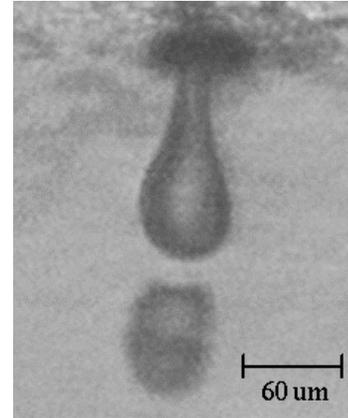
Figure 3: Water droplet ejection through 60 μm diameter orifice by using the large-scale device
