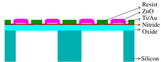
Patterning photoresist layer for top electrode layer liftoff
