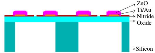
DC planar reactive magnetron sputtering of 0.4 microns ZnO
