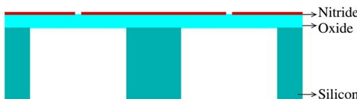
Patterning 8 microns holes in the nitride by dry etch
