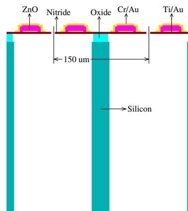
Figure 1: Side view of two adjacent elements of the developed micromachined two-dimensional array of ejectors
