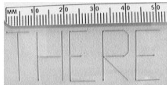
Figure 4: Drop-on-demand direct write with photoresist by using the large-scale device: the lines are 350 μm wide
