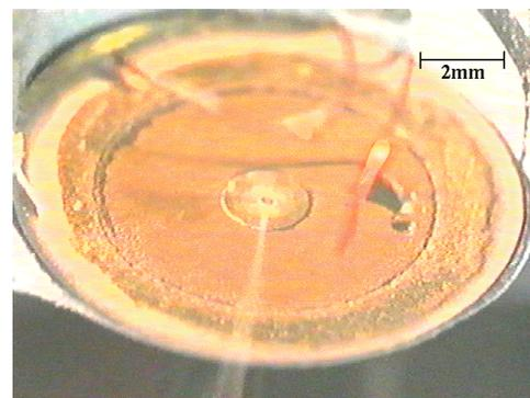
Figure 5: Small solid particle ejection through 150 μm orifice at 2.9 kHz
