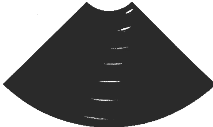
Fig. 7 Reconstructed image of a six-wires phantom at 30 dB signal-to-noise ratio.
