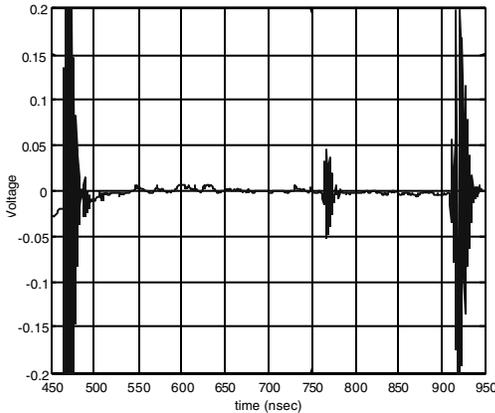
**Figure 6. Reflections from the top of the channel filled with DI water.**
