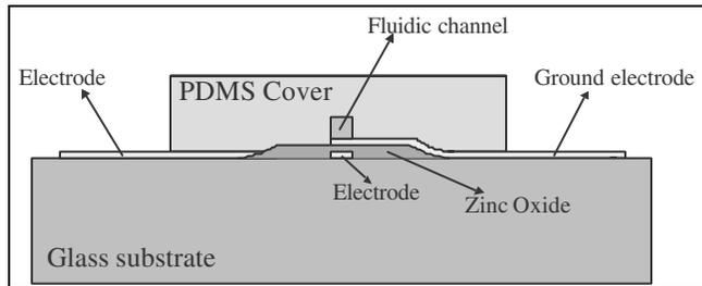
Figure 2. A cross-section of the micro-fluidic device.
