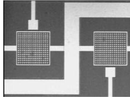
**Figure 11. A picture of a cMUT device for micro-fluidic applications.**
