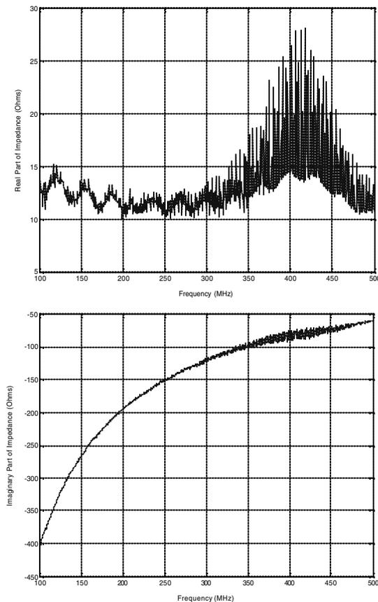
Figure 3. Impedance of ZnO transducer.
