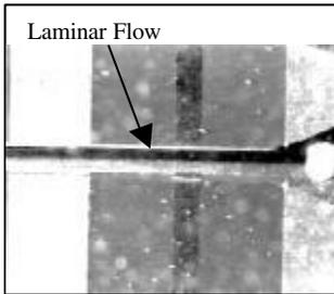
**Figure 9. Laminar flow of two fluids in a micro-fluidic channel.**
