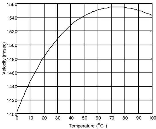
**Figure 7. Velocity of sound in DI water as a function of temperature.**
