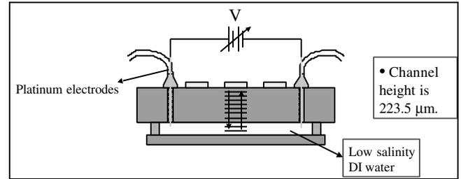
**Figure 8. The experimental setup for temperature measurement.**
