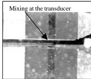
**Figure 10. Mixing of the two fluids at location of the transducer.**
