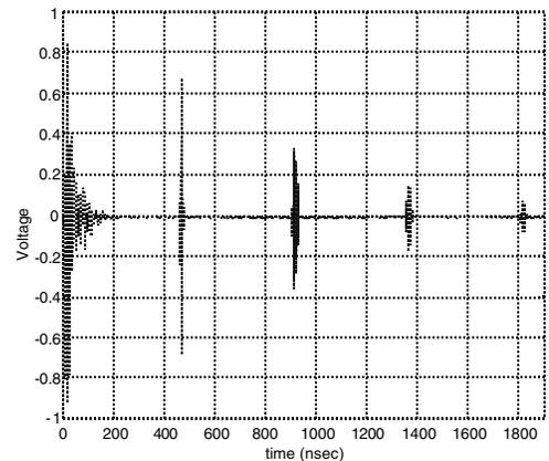
Figure 5. Reflections from the glass substrate.
