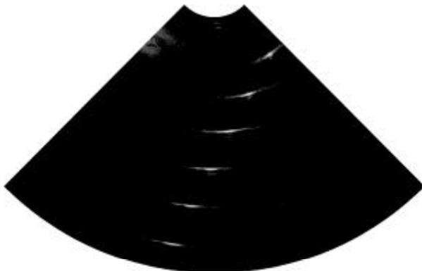
**Figure 8: B-scan sector image using 64 element 1D cMUT array. Display dynamic range is 50 dB.**
