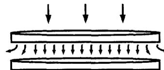
Figure 5: A representation of squeeze-film damping between two parallel plates in air
