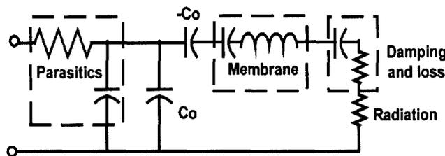
Figure 4: Equivalent electrical model of a transmitting CMUT in air
