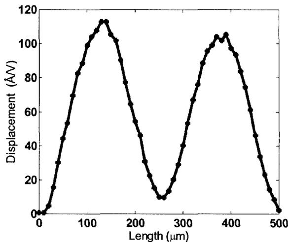
Figure 8: Unexpected second-order mode shape across length of a rectangular transducer
