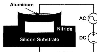
Figure 1: Schematic cross-section of a single CMUT membrane
