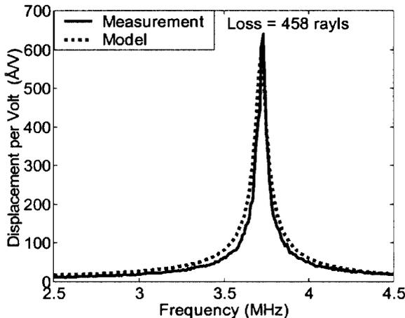
Figure 6: Measured displacement per volt across the transducer by frequency, compared to the prediction by the equivalent circuit model
