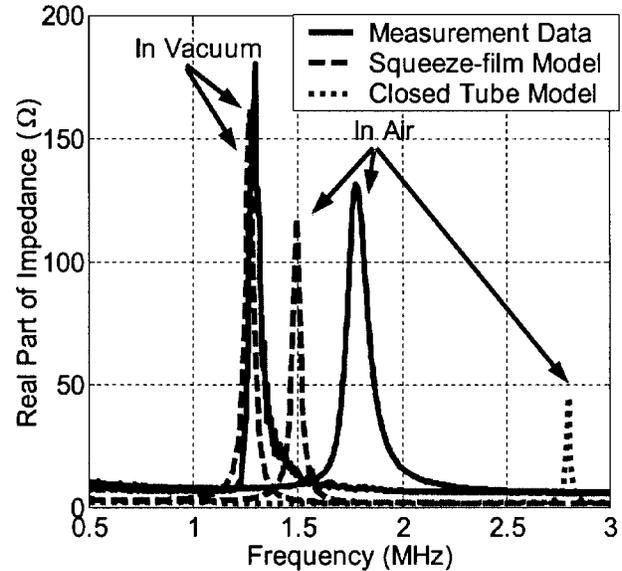
Figure 7: Real part of impedance in vacuum and air comparing predicted frequency-shift of the squeeze-film model and closed-tube model with the measurement
