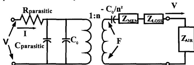
Figure 3: Model of a transmitting CMUT in air
