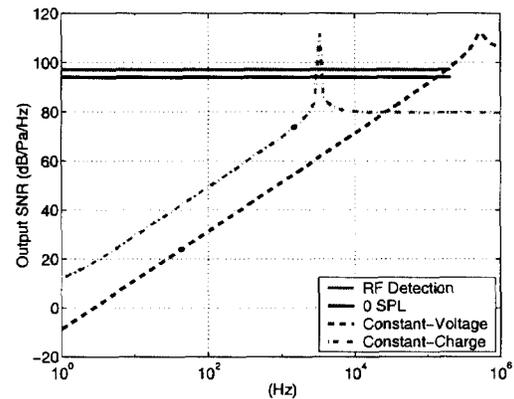
Fig. 6. Output SNR of a 1 mm<sup>2</sup> device.
