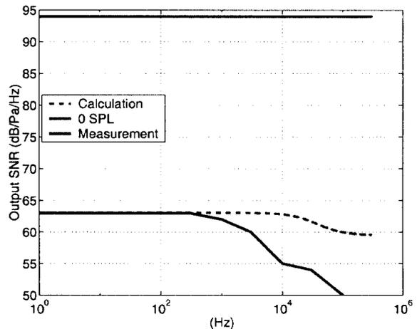
Fig. 10. Measured SNR of the microphone compared to 0 SPL.
