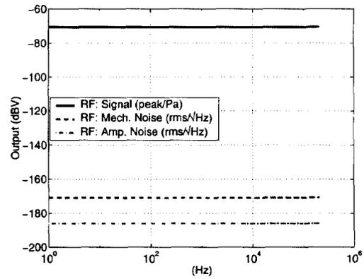
Fig. 5. Output signal and noise levels of a 1 mm<sup>2</sup> device with RF detection.
