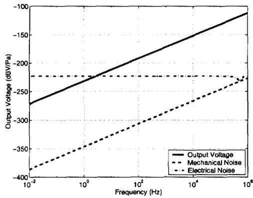
Fig. 3. Output signal and noise levels of a 1 mm<sup>2</sup> device under constant-voltage regime.
