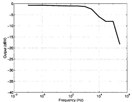
Fig. 9. Frequency response of the microphone.
