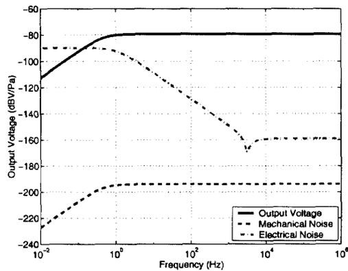
Fig. 4. Output signal and noise levels of a 1 mm<sup>2</sup> device under constant-charge regime.
