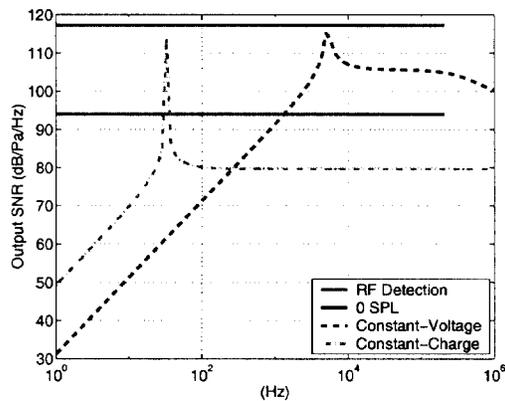
Fig. 7. Output SNR of a 1 cm<sup>2</sup> device.
