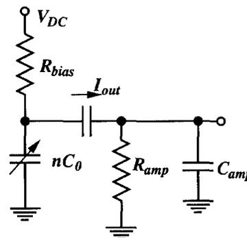
Fig. 2. Traditional detection circuitry.
