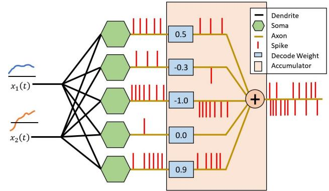
Fig. 1. Braindrop Spiking Neural Network Architecture
