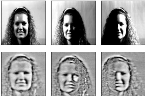
Fig. 9. CCD Camera (top row) versus retinomorphimic imager (bottom row) under variable illumination. The CCD camera has global automatic gain control (AGC), whereas the retinomorphimic imager has local AGC and performs bandpass filtering.
