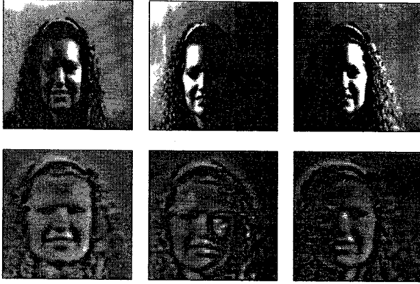
Figure 5. CCD Camera (top row) versus OPL imager chip (bottom row) under variable lighting. The CCD camera performs global AGC whereas the OPL chip performs local AGC and bandpass-filtering.
