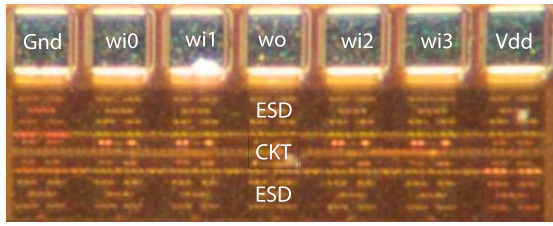
Fig. 7. Receiver Pads ( 271.4\mu\text{m} height; 100\mu\text{m} pitch). All logic circuitry (CKT) resides in the enable pad—taking up less than 75 \times 13\mu\text{m} ( 0.18\mu\text{m} process)—sandwiched between electrostatic discharge devices (ESD).
