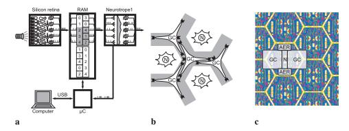
Figure 2: **a.** Neurotrope1 system. Spike communication is by address-events (AER). **b.** Neurotrope1 cell mosaic. The extracellular medium (grey) is laid out as a monolithic honeycomb lattice. Growth cones (GC) occupy nodes of this lattice and extend filopodia to the adjacent nodes. Neurotropin receptors (black) are located at the tip of each filopodium and at the growth cone body. Target cells (N) occupy nodes of an interleaved triangular lattice. **c.** Detail of chip layout.
