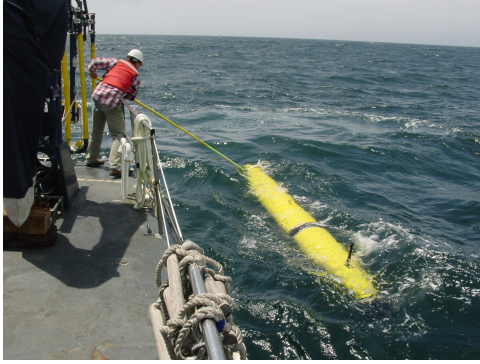
Figure 1: Picture of retrieval of the MBARI Dorado mapping AUV. ©MBARI.
