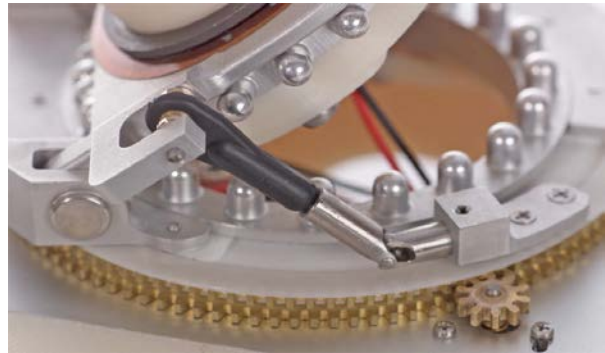
Figure 4: Elevation Arm in CubeHATTS Prototype
