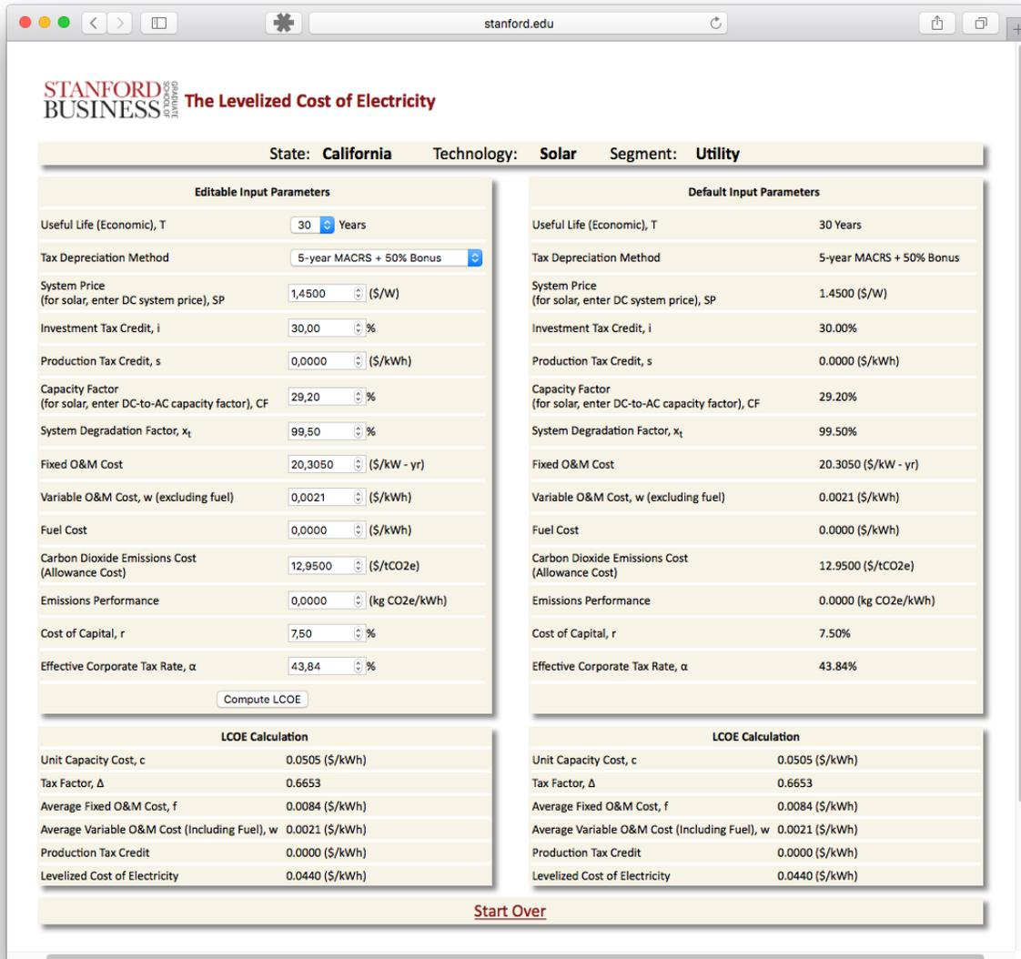
Figure 2: Result and parameter page of the LCOE Calculator.
